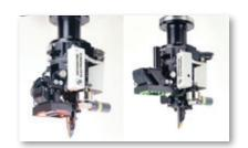
Non-Destructive Pulltest gives 100% physical testing of the bonds after they are made which in turn offers real-time quality physical control
