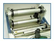
Automatic reeling and removal of UV tape backing
