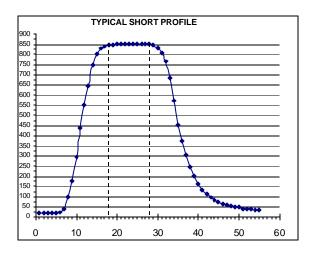
at a peak temperature of 850?C recommended. Air flow rates must be optimized to ensure that the products of binder burn-off discharge properly and create a fully oxidizing atmosphere in the muffle.
