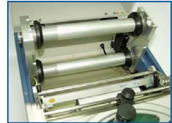
*Automatic reeling and removal of UV tape backing*
