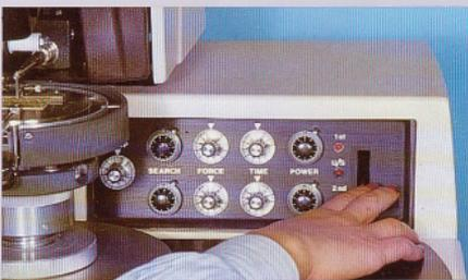
**Individual dial setting** of 5 parameters for 1st bond and 2 bond : bonding time, bonding power, bonding force, search height, and loop height.
