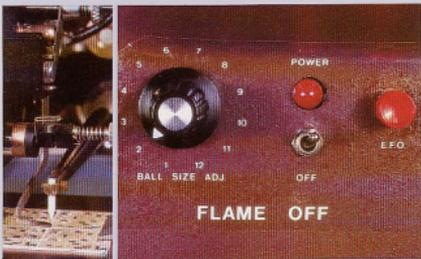
Electronic flame-off system offers handy adjustment of ball size and clean harmless ball formation, covering the entire wire size range.
