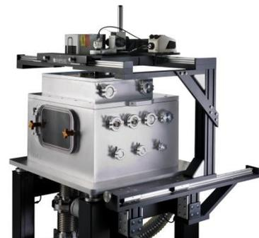
Built on a vibration isolation table, the chamber contains the wafer stage, the chuck system with carrier plate and manipulators. The motorized/programmable wafer stage provides up to 205 mm x 205 mm of X, Y movement and has motorized/programmable Z and theta stages. Several thermal chuck options are available to provide temperature ranges from -60°C to 300°C.
