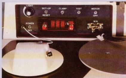
Dual operation mode allows either chessman or manual Z control (optional) for precise bond placement and more flexibility in multiple-bonding-height devices.
