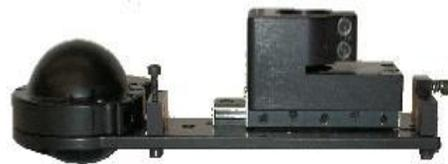
The third option for holding and positioning the integrating sphere on these systems utilizes a unique manipulator mount. This manipulator mount also enables the user to quickly configure for either EELD or VCSEL applications. In addition, this unit is designed to swing up out of the way for loading and then return to the precise spot where it was originally aligned. Most VCSEL test applications only require a less expensive StereoZoom microscope to consistently obtain precise, meaningful data.
