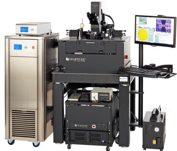
SA-8 semiautomatic probe system with a -65°C to 300°C thermal chuck, localized environmental chamber, compound optics, HF manipulators mounted on a vibration isolation table - several configurations available.
