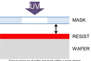
Typical exposure of wafer and mask within a mask aligner.
