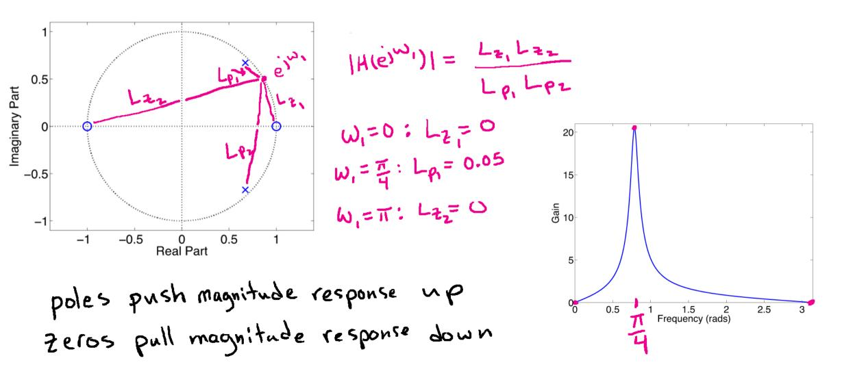
Can infer filter characteristics from pole/zero plot
