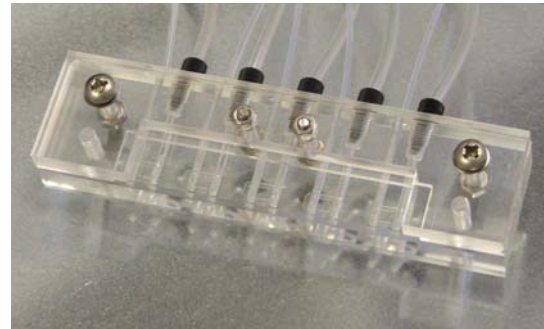
Figure 3.6 A 5-parallel flow-cell cytometry device incorporating micro- and milli-fluidics. Housings such as this are fabricated by INEX using its in-house CNC micro-milling capability.
