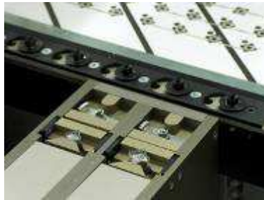
Nicomatic metal dome feeder
