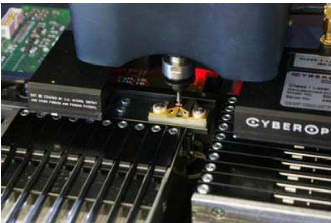
Measuring station, installed on tool changer
