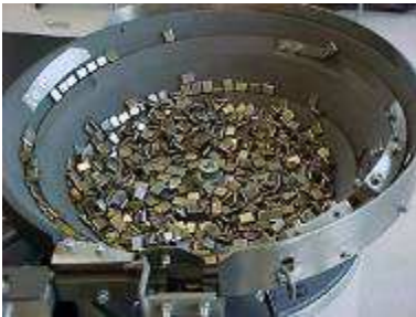
Vibratory bulk feeder
