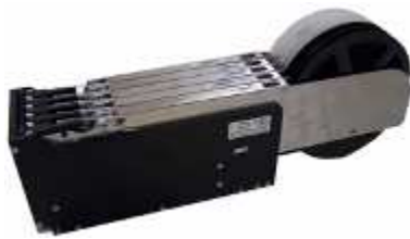
CLM941 or CLM942 adapter with single feeders
