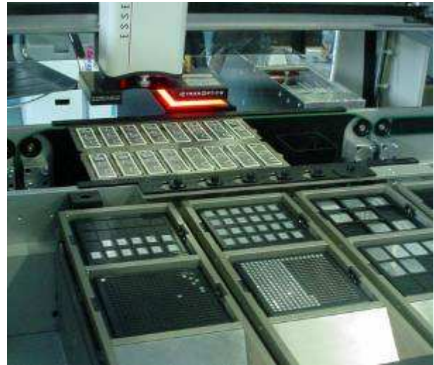
Tray stack feeding system for chip on board applications
