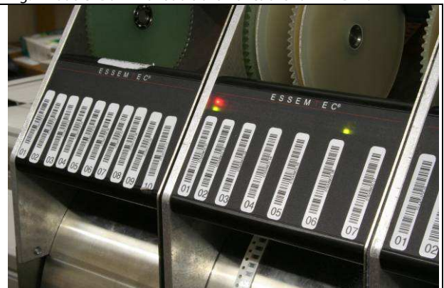
Fig. 4 Each feeder slot is marked with a barcode.
