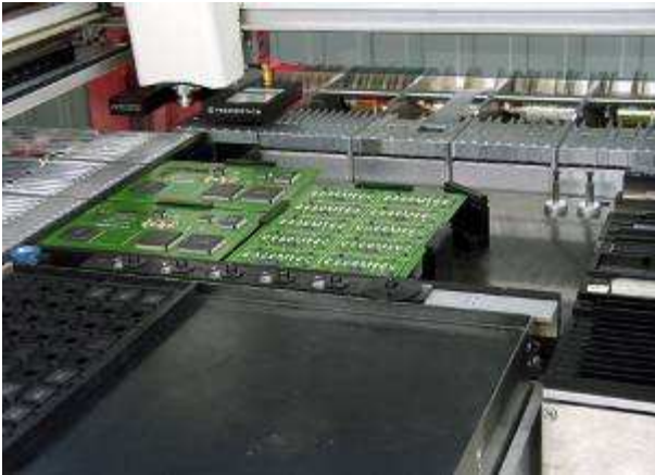
Standard magnetic PCB holder (FLX2011)
