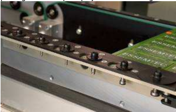
Tool changer with pneumatic safety lock.
