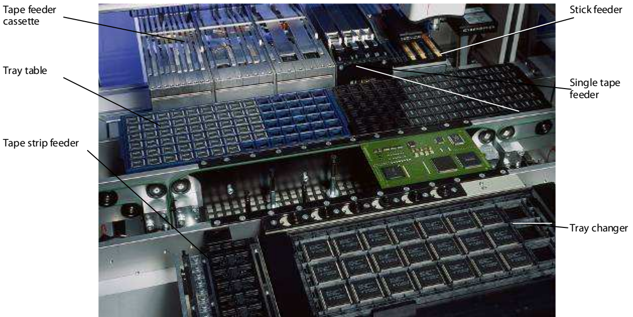
Tray stack feeding system for chip on board applications
