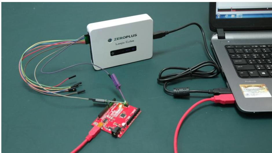
**Figure 2-1 Hardware connections**
