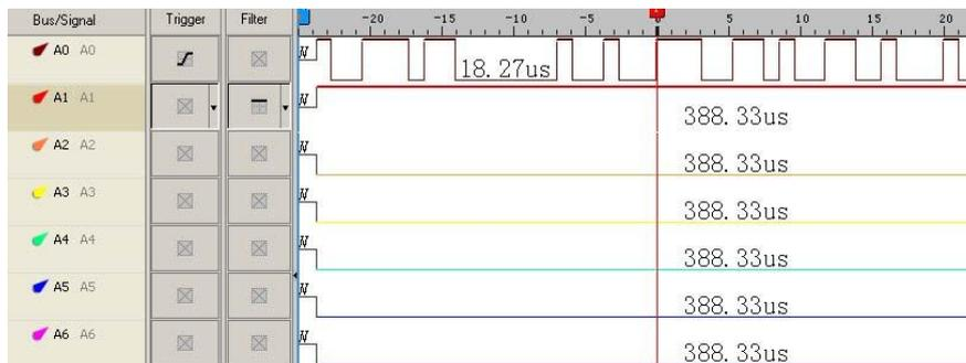
Figure 4-33 Signal Filter example / Post-filter signal with A1 filter = High
