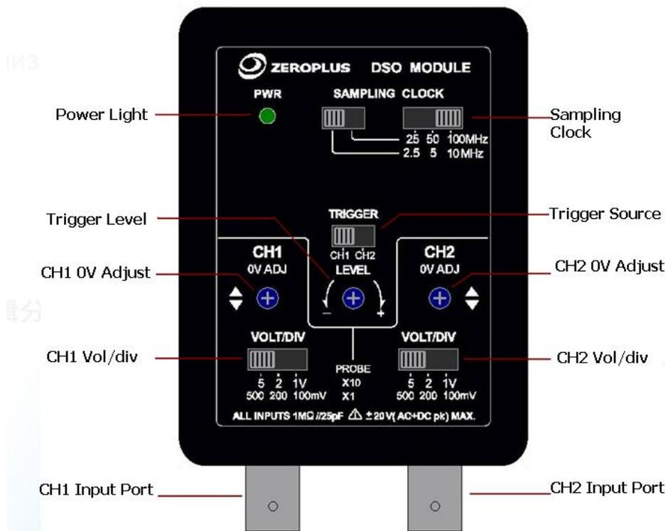
Figure 4-107 DSO Module Setting Panel
