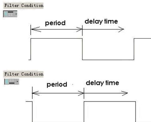
Figure 4-31 Signal Filter / Delay Start Point – Period + Delay
