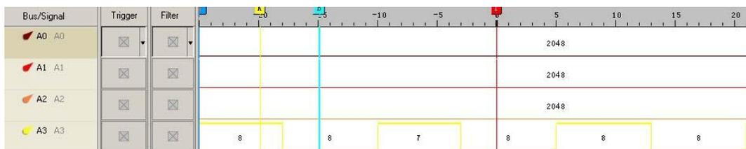
Figure 4-75 Noise filter example / After applying 5 clock filter
