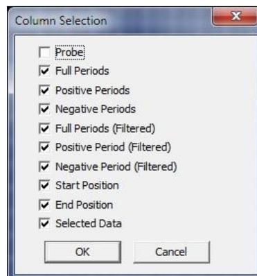
Figure 4-98 Statistics / Customize – Select which columns to display
