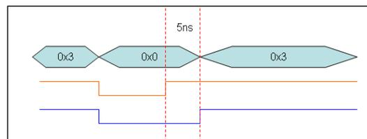
Figure 4-72 Bus Width Filter example – After applying filter
