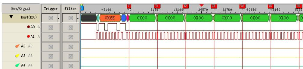
Figure 4-41 Protocol Analyzer Trigger Mark
