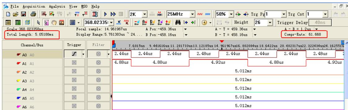
**Figure 4-27 Ex: Acquisition with compression – 5.05188ms acquisition**
