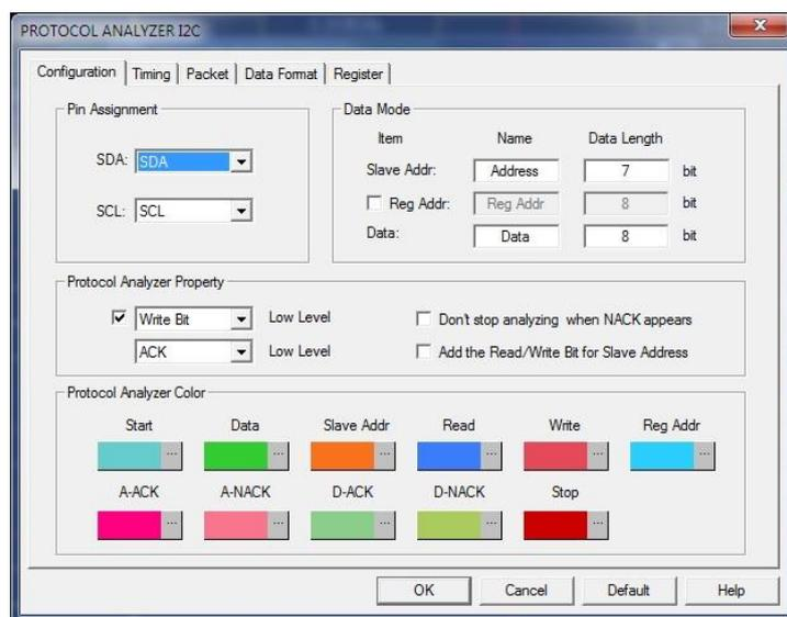
**Figure 4-21 Protocol decoder I2C configuration dialog box**
