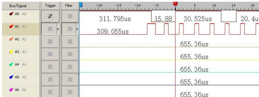
Figure 4-32 Signal Filter example / Pre-filter signal
