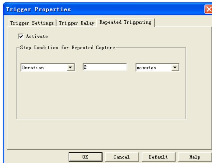
Figure 4-46 Repeated Triggering dialog box
