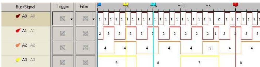
Figure 4-74 Noise filter example / Before applying 5 clock filter
