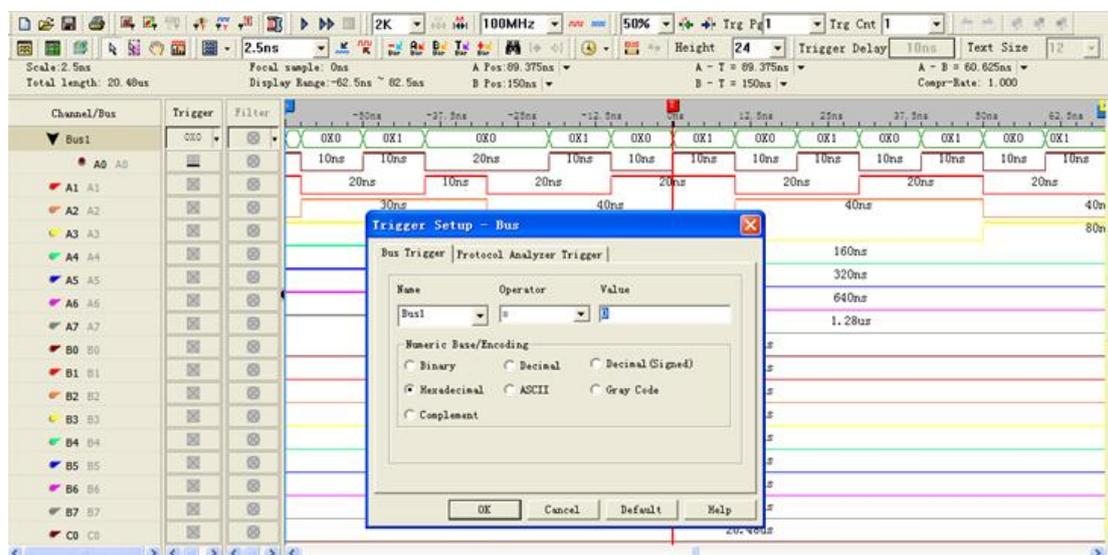
**Figure 4-37 Bus Trigger example**
