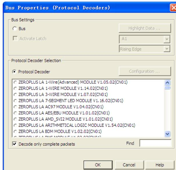
Figure 4-20 Bus properties (Protocol decoders) dialog box
