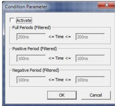
Figure 4-99 Statistics / Filter – Apply filter conditions
