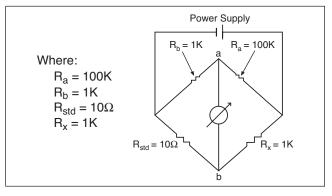
We used a basic Wheatstone bridge circuit. The resistance values of the arms of the bridge were selected to place a high power on the test resistor  $(R_x)$ , while ensuring a very low power on the three remaining legs. When the power is increased, any deflection in the null meter between points a and b is attributed to the self heating of  $R_x$ .
