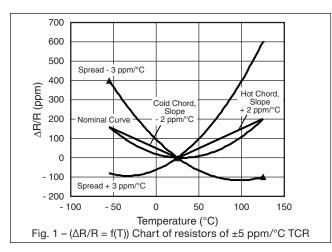
corresponding to a TCR of—and +2 ppm/°C and two curves corresponding to a spread of—and +3 ppm/°C from the nominal.
