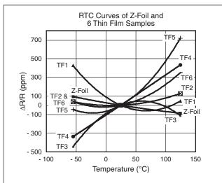
Fig. 9 – Relative resistance change vs. temperature curves of Z-Foil and thin film precision chip resistors from 6 vendors
