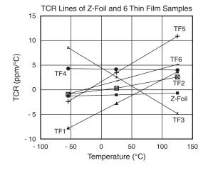
Fig. 10 – Temperature coefficient of resistance as function of temperature of resistor chips per Fig. 7
