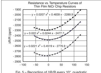
Fig. 5 – Recording of  $\Delta$ R/R every 10°, quadratic trendlines and equations of three NiCr thin film chips.
