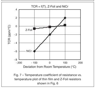
the thin film resistor's TCR changes between -2 ppm/°C and -8 ppm/°C, while the Z-Foil's from -0.2 ppm/°C to -0.8 ppm/°C only.
