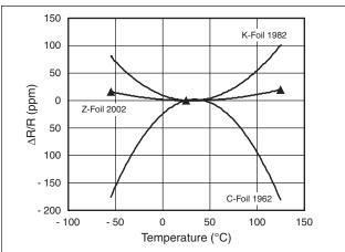
Fig. 4 – Three resistance vs. temperature characteristics of foil resistors and year of their introduction.
