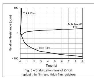
The key to high speed of the thermal step function are a low thermal time constant and a low resistance change,  $\Delta R/R$ , due to the Joule effect. This can be achieved by using resistors of low TCR (see Fig. 8).
