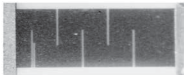
Figure 2. Blank image, laser trimmed. Final trim performed by a second cut in the left kerf. It can provide between 1.66 and 20 squares of resistance.
