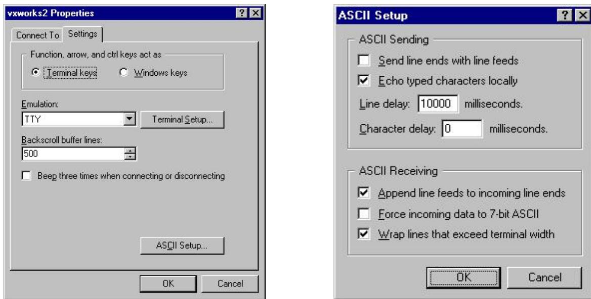
With Hyper-Terminal, an ASCII text request message can be sent to VIP-9-SIO and an ASCII text response can be displayed on the Hyper-Terminal window.
