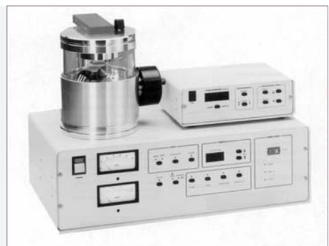
The rotary planetary stage with tilt ensures that highly contoured samples are evenly coated. This ensures that the minimum coating thickness can be applied to give conductivity without compromising fine specimen detail. The dual height 150 mm diameter work chamber gives easy adjustment of working distance.
