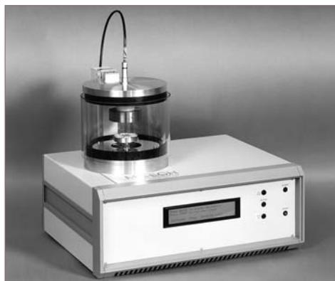
This is a simple, free-standing glow discharge system, typically used for hydrophobic to hydrophilic conversion of carbon coated TEM grids thus allowing easy spreading of aqueous suspensions. The unit requires only a suitable rotary pump for operation. It has intuitive digital menu-driven operation which makes it easy to set up and run. For ultimate safety the system has a built-in implosion guard.
