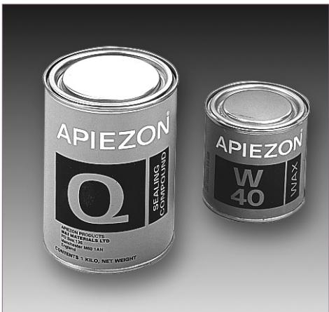
Apiezon® W is a low vapour pressure wax for sealing joints in high vacuum pressure systems. It has a working temperature range of -10 to 75 °C. It is the most resistant to attack by acids and alkalis, has the lowest vapour pressures and is the most resistant to water.
