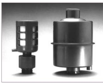
Filters are available for the removal of oil mist from vacuum pump exhaust gases. The units are disposable and must be fitted vertically. Each unit consists of a microfibre element permanently sealed into either a nylon housing with  $\frac{1}{2}$ " NPT male fitting suitable for a flow rate up to 5 m<sup>3</sup>/hour (83 l/min), or a steel housing with  $\frac{1}{3}$ " NPT fitting suitable for a flow rate up to 15 m<sup>3</sup>/hour (250 l/min). Other sizes available on request.
