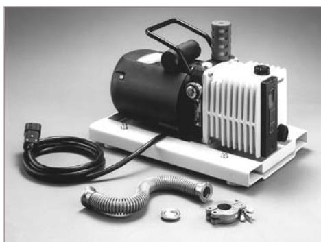
This compact pumping system is designed for use with Agar coating units. The 2.5 m<sup>3</sup>/hr two-stage rotary pump is mounted on an anti-vibration platform and is equipped with an oil mist filter. The metal bellows with KF fittings provides a short, wide bore connection for maximum pumping efficiency. Pump down time to 0.1 mbar is 30 seconds.
