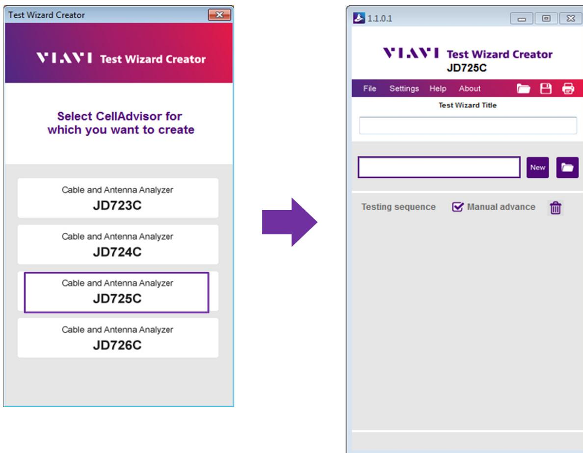
Caution: Test wizard and testing unit files that you create can work only for the particular model you select.
