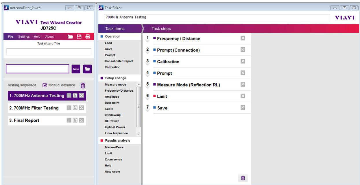
In Test Wizard Creator, there are two elements that you need to be familiar with: **testing units** and **tasks**. You can create your test wizard with one or multiple testing units in the [main window](#) and then define each testing unit with many specific tasks in the [task editor window](#), depending on your needs.
