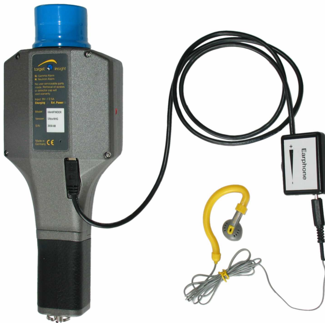
Figure 24 Connection of earphones to the identiFINDER
