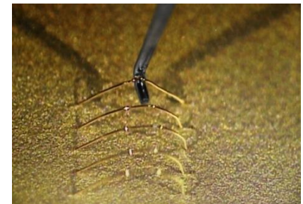
pull test with hook
