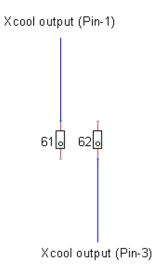
Output Pin 1 of the Xcool must be connected to terminal X1:61 (upper row) and output Pin 3 to terminal X1:62 (lower row). Therefore, the bridge between X1:61 and X1:62 must be removed.
