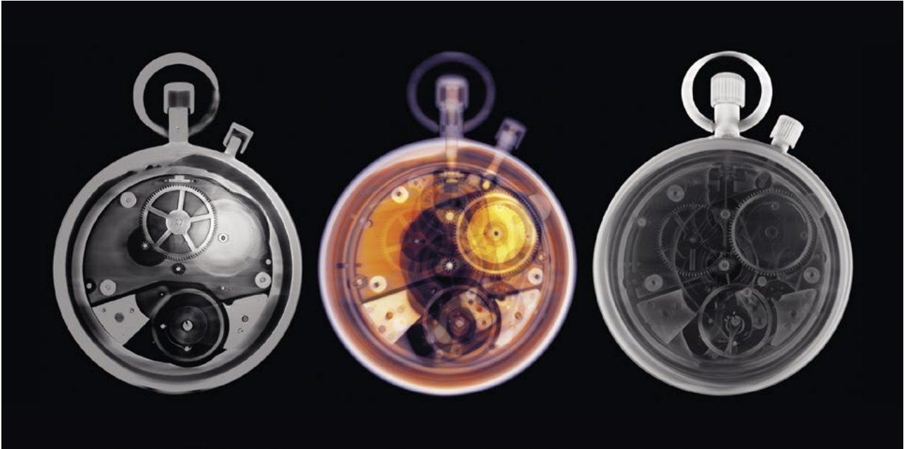
CT reconstruction and 3D volume visualization of a watch
