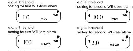
Although the dual alarms are referred to as first WB and second WB the EPD will operate correctly even if the second WB alarm thresholds are set lower than the first WB thresholds.
