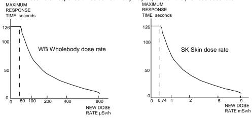
e.g. if the WB rate changes to 50  $\mu$ Sv/h, the maximum time the Dosemeter takes to respond fully to this change is 126 seconds. The calculated rate changes roughly linearly towards the correct rate over this time period except when a large fall in rate is seen. In this case the response is rapid at first, before becoming roughly linear.
