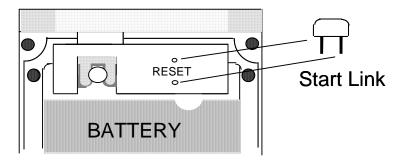
If the display does not appear check that the battery has been fitted correctly. If the battery feels warm remove it immediately as it may have been short circuited. This battery should be replaced in the Polythene bag from where it came and allowed to cool in a safe place.
