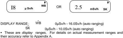
Over-range is indicated with a continuous alarm and a flashing LCD display - see section 2.5.5.
