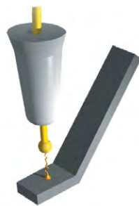
Consistent EFO firing to form consistent free-air ball
