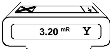
To change position of decimal point and to change Rad unit (microRem or milliRem), press indicated button.
