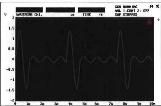
Fig. 3: The waveform function displays the test signal in the time domain. The example shows a sine wave burst
