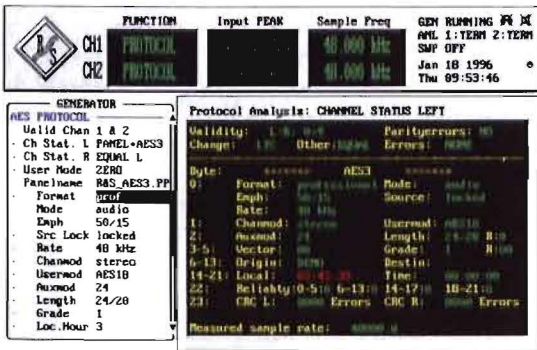
Fig. 12: UPL generates and analyzes additional data in digital data streams in line with all common standards. The data are represented in binary form, as hexadecimal numbers, as ASCII characters or evaluated in consumer or professional format
