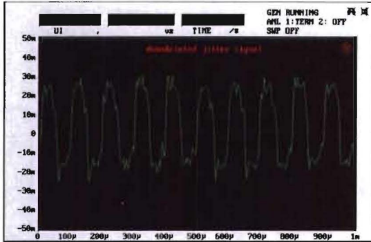
Fig. 10: Display of jitter signal in time domain
