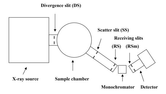
The sample height is very important when a focusing geometry is used. The correct sample height is given by the vertical flat surface inside the sample chamber.
