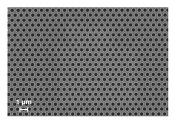
Figure 2: Array of holes on a hexagonal lattice printed on the PhableR 100 system. Hole period and diameter are 600nm and 300nm, respectively.
