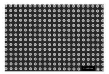
Figure 1: Precisely fabricated dot matrix using Displacement Talbot Lithography principle. Dot period and diameter are 300nm and 140nm respectively.
