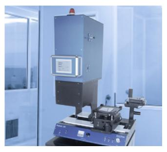
Figure 4: PhableR 100 Displacement Talbot Lithography System
