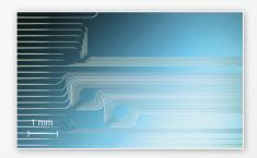
Multiple mm-length tapered waveguide array R. Schmits, TNO Delft
