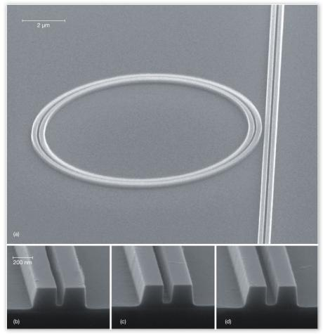
Waveguide coupling device with critical gap control Courtesy: Linjie Zhou, Katsunari Okamoto, and S. J. Ben Yoo, University of California Davis, and James Conway, Stanford Nanofabrication Facility
