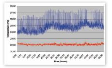
No impact on system demonstrated by artificial fluctuations of room temperature
