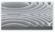
Fresnel lense array in 5 µm thick resist
