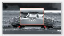
Two T-gates (viewed in cross-section) are located under electroplated airbridge
