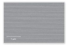
UHR crossection: 11 nm lines in PMMA
