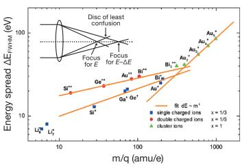
Figure 7: Energy spread and chromatic aberration of AuGeSi and GaBiLi LMAIS
