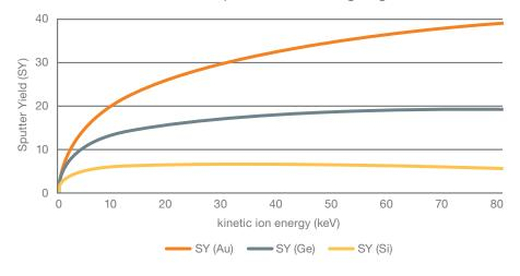
Figure 12: AuGeSi sputter yield as a function of ion energy
