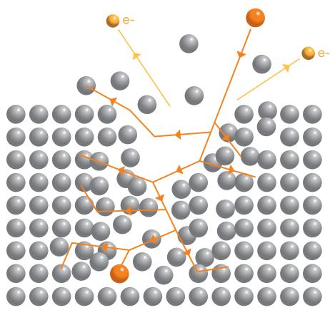
Figure 2: Ion beam and substrate interaction. Impacting ions generate electron and ion emission and are finally implanted into the substrate
