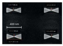
Figure 11: Stepwise fabrication of bowties/50 nm Au on Si substrate
