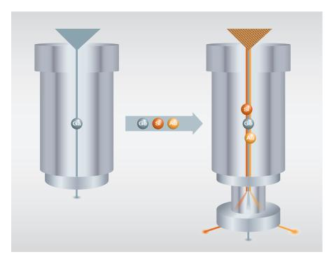
Figure 1: Schematics of nanoFIB column for Ga FIB (left) and nanoFIB with IONselect extension including LMAIS and Wien filter (right)
