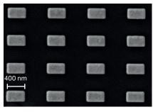
b) Step 2: Li FIB for fine shaping of rectangular boxes to fabricate bowtie structures at highest resolution
