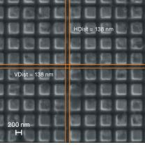
Figure 13: Illustration of the milling strategy on a functional film of a layered sample to avoid contamination of the silver layer was milled using the Au ion beams to speed up the process, as the sputter yield is 5 times higher compared to Si. The remaining 20% of the layer was cleaned up using Si<sup>++</sup> to avoid contamination of the Si<sub>3</sub>N<sub>4</sub> layer.
