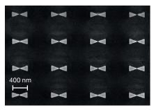
c) Li FIB adjustment of the gap size of the bowtie nanoantenna
