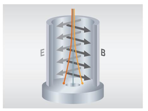
Figure 4: ExB filter setup to separate ions of different mass and charge
