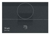
Automated metrology and statistical evaluation for both LER and a single distance measurement for gap determination – all applied to 135 devices exposed at different places
