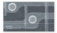
Large-area high-resolution mosaic image of an IC, free from visible stitching errors. The white lines indicate the stitching borders.
