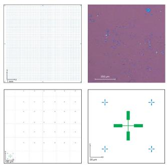
Figure 1 Fiducial marks on substrate with randomly distributed graphene flakes
