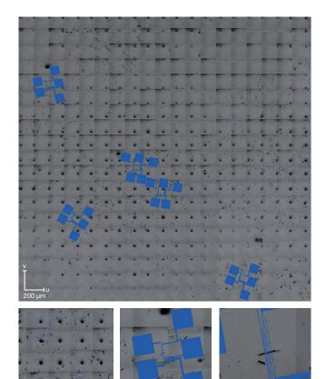
Figure 3 Aligning electrode patterns onto large area SEM image to functionalize selected graphene flakes
