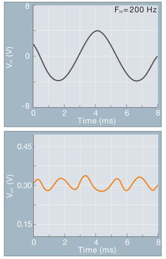
Figure 11 AC input signal (top) and measured output waveform (bottom) of the fabricated graphene frequency tripler
