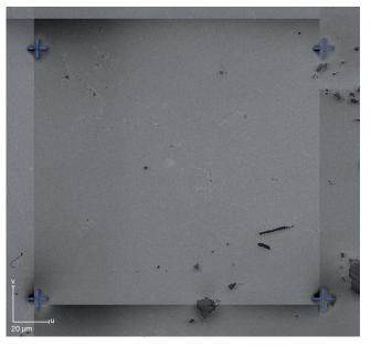
Figure 2 SEM image of fiducial marks and graphene flakes
