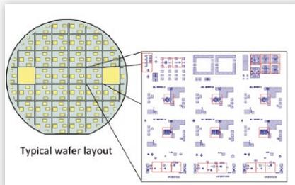
Chip layout with Writing Fields (WFs) positioned according to gate positions
