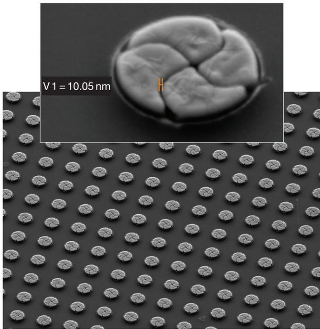
**Figure 5:** Tilted SEM view of a 25 μm x 25 μm gold nano-disk array with 1 μm period. The inset shows a single disk with 500 nm diameter including a sinusoidal low-dose cross cut with 10 nm gap.
