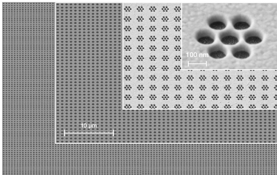
Figure 6: Oligomer Structures with Heptamer-arranged nanohole arrays<sup>13</sup>
