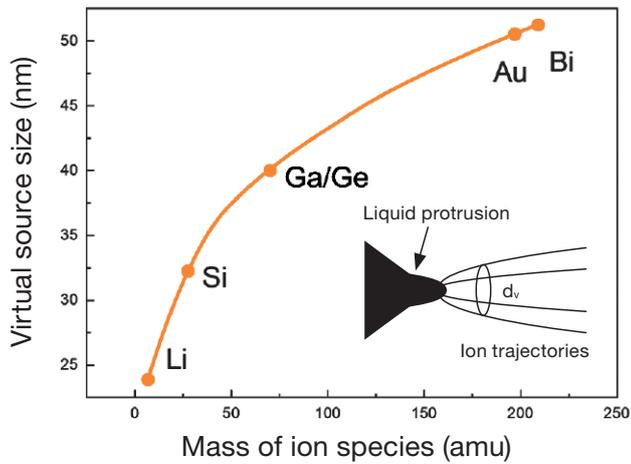
Figure 6: Virtual source size depends on ion mass, therefore light ions have a small virtual source size ( $d_v$ )
