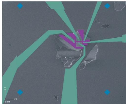
**Figure 8:** Electrodes and etch mask definition
