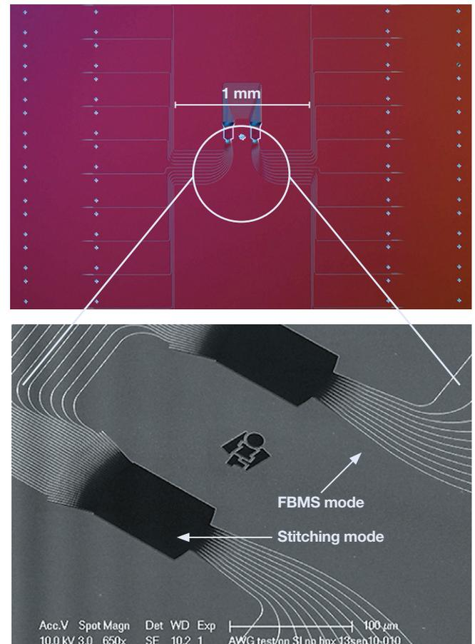
**Figure 1:** An arrayed waveguide grating (AWG) over several mm length. Courtesy R. Schmits et al., TNO Delft, Netherlands.
