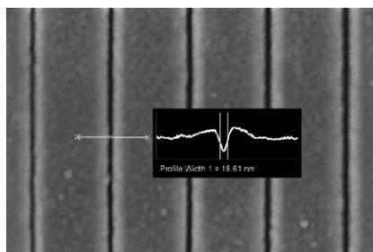
Figure 15: 19nm Au ion beam for Au layer
