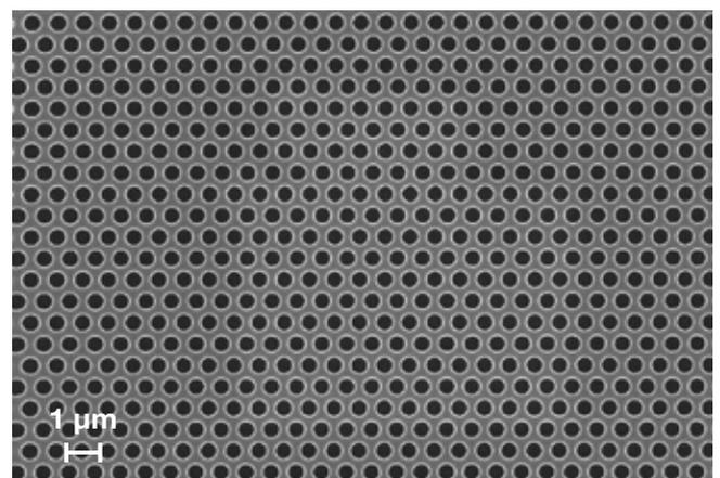
**Figure 2:** Array of holes on a hexagonal lattice printed on the PhableR 100 system. Hole period and diameter are 600nm and 300nm, respectively.
