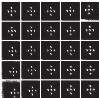
Figure 2: Write field before corrections; stigmatism and distortions may harm stitching performance
