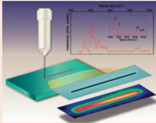
**Schematic representation of an example of an FIB-directed growth process. After patterned ion implantation and subsequent annealing of the SiC sample, graphene grows only in the implanted regions.<sup>1</sup>Image courtesy of Brent Gila**
