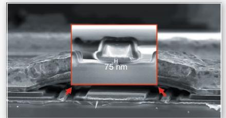
Two T-gates (viewed in cross-section) are located under electroplated airbridge
