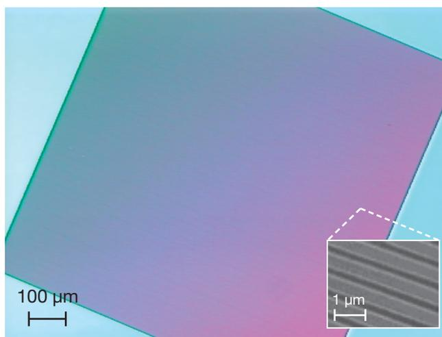
**Figure 8:** Optical microscope image ( $\times 10$ ) of a  $1 \times 1 \text{mm}^2$  large area grating with a pitch of 0.7  $\mu\text{m}$  and rotated by  $20^\circ$ , showing no visible stitching boundary.
