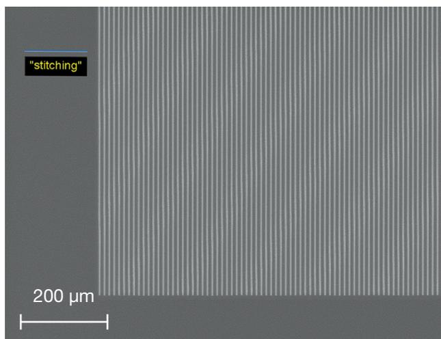
**Figure 7:** Area grating with a pitch of 1  $\mu\text{m}$ , fabricated by “stitching” of 50  $\mu\text{m}$  wide strips patterned by MBMS.
