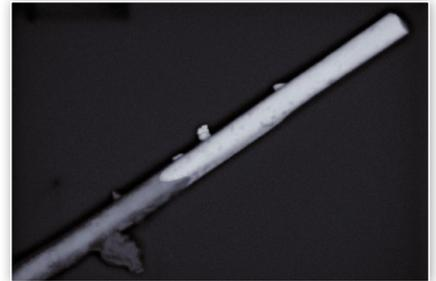
Compositional / material contrast showing an Au-capped Ni/NiO<sub>2</sub> nanowire, clearly resolved with inlens EsB detector
