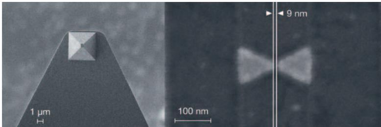
**Plasmonic nano-antenna on top of a gold-coated AFM tip. Direct milling, *ie* without the need for using a resist, enables high-resolution features even on topographic samples. Image produced by Raith for Professor Moerner, Stanford University, USA**
