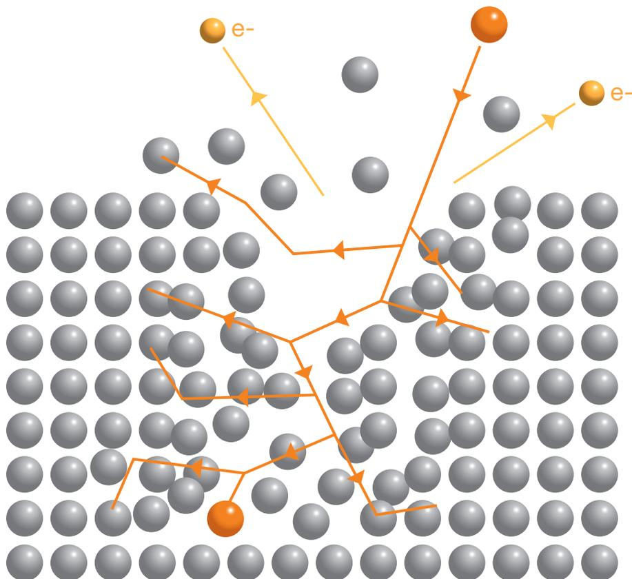
Figure 2: Ion beam and substrate interaction. Impacting ions generate electron and ion emission and are finally implanted into the substrate
