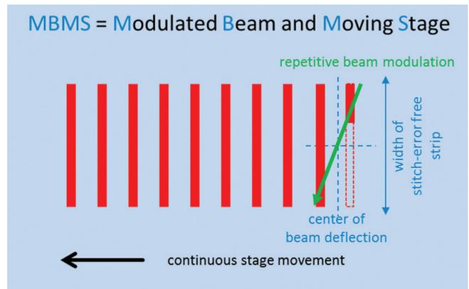
**Figure 2:** Principle of Modulated-Beam-Moving-Stage: Continuous stage movement with repetitive beam modulation, resulting in stitch-error-free strips with a length of several mm or even cm.
