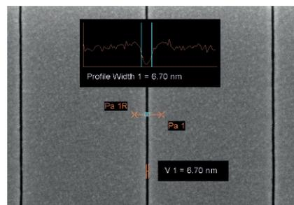
Figure 4: Minimum feature size obtained in a bulk sample. Gallium milling of a Chromium layer on silicon substrate, line width < 10 nm
