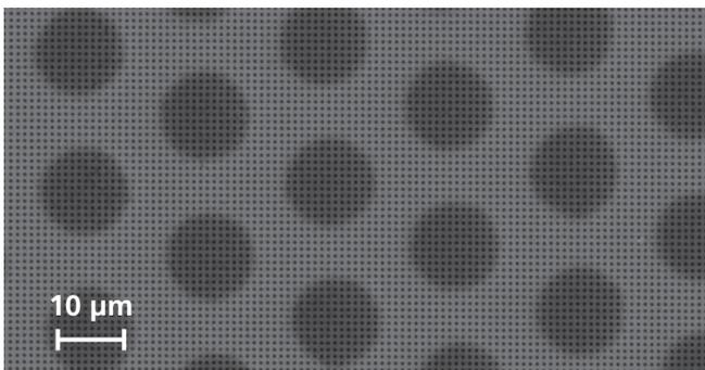
**Figure 12:** Nanosieve with periodic holes<sup>[5]</sup>.
