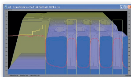
▲ Photonic crystal exposure optimization using NanoPECS proximity effect correction package a) with the help of 3D resist development simulation for identification of critical areas b) with the help of proximity corrected dose distribution. ►
