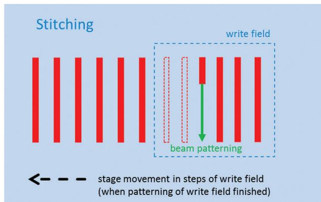
**Figure 4:** Illustration of conventional stitching mode: Beam deflection and subsequent stage movement.
