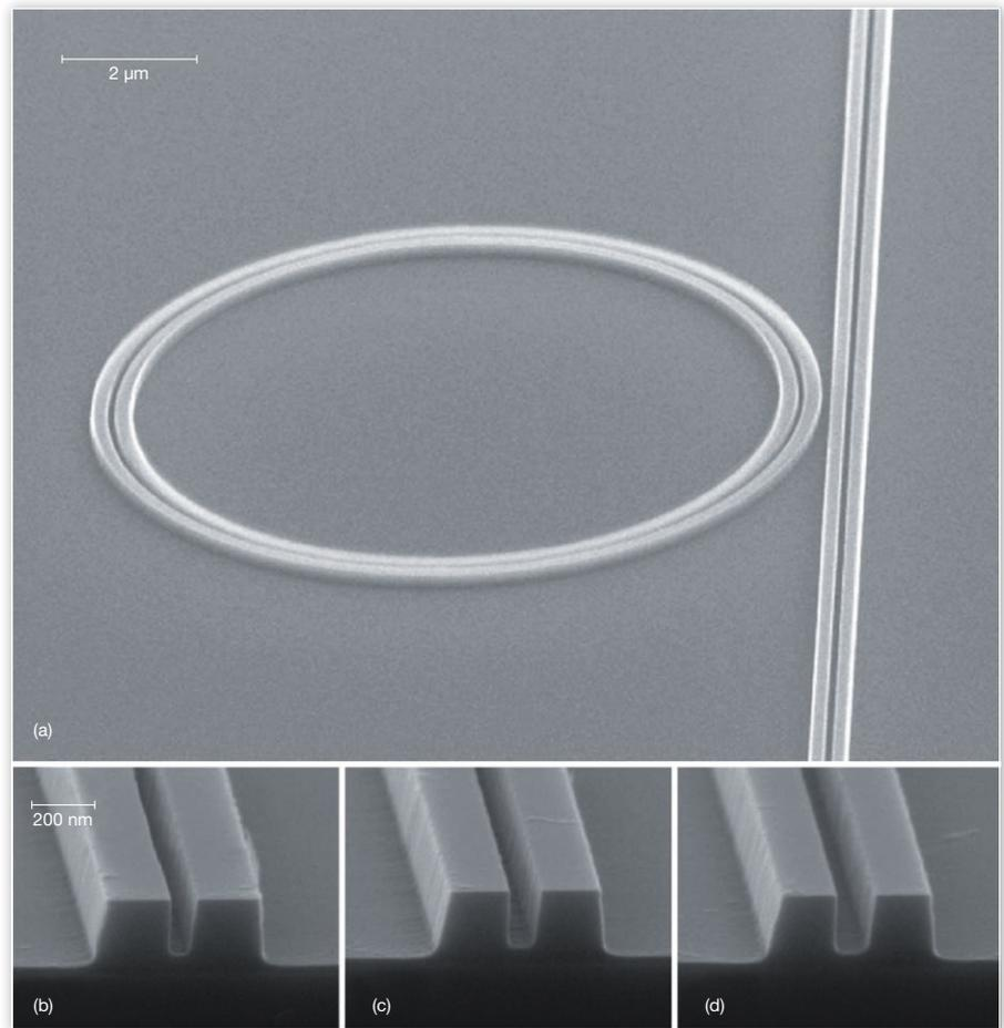
Waveguide coupling device with critical gap control
