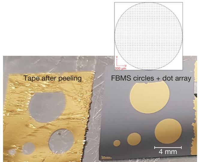
**Figure 7:** Photograph of gold circle sample, tape after stripping and FBMS circle design including dot array.
