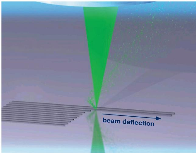
**Figure 2:** Illustration of conventional stitching mode. The beam is deflected while the stage is stationary, resulting in stitching errors of some nm.
