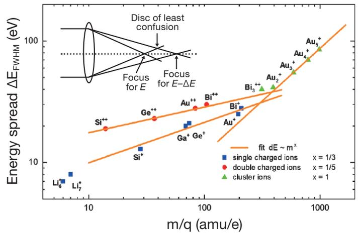
Figure 7: Energy spread and chromatic aberration of AuGeSi and GaBiLi LMAIS
