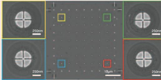
Array of precisely and reproducibly patterned gold nanoparticles for plasmonics applications. Reprinted with permission from Gervinskas G, Seniutinas G, Rosa L, Juodkazis S. Arrays of arbitrarily shaped nanoparticles: overlay-errorless direct ion write. *Advanced Optical Materials* 2013;1:456-9 ©Wiley-VCH Verlag GmbH & Co.<sup>1</sup>
