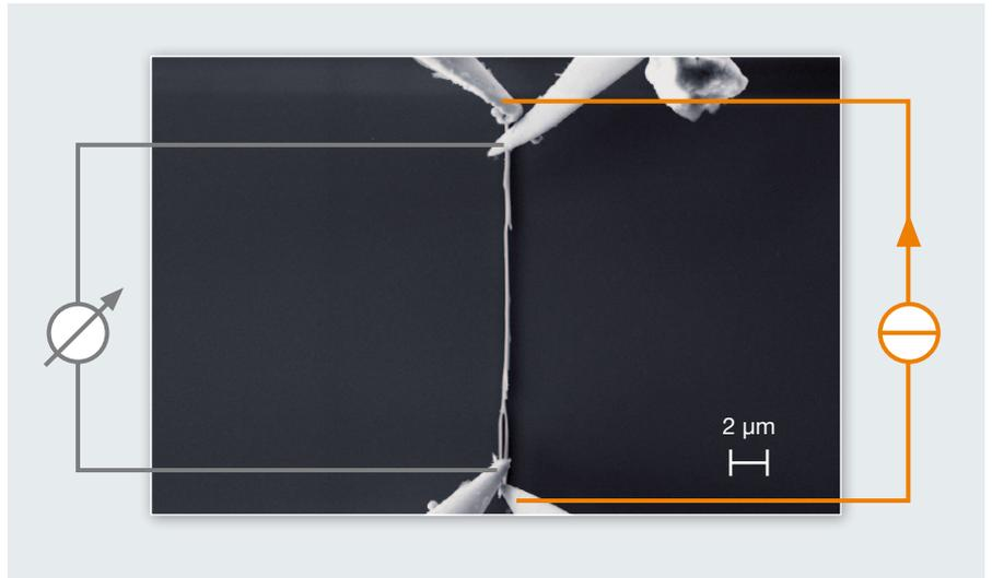
Direct-contact nanoprobng (4-point electrical measurement) of a Ni/NiO<sub>2</sub> nanowire with Au-caps
