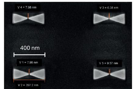
Figure 11: Stepwise fabrication of bowties/50 nm Au on Si substrate
