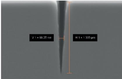
Figure 10: X-section of cleaved substrate perpendicular to a 1mm-long line, GaAs
