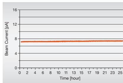
Figure 12: Probe current of Raith's LMAIS showing excellent long-term stability suitable for most nanofabrication tasks
