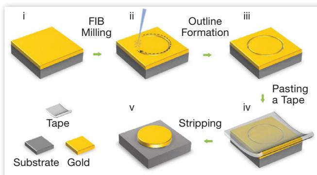
**Figure 1:** Principle of Sketch & Peel<sup>[2]</sup>.
