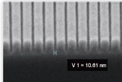
UHR crosssection: 11 nm lines in PMMA
