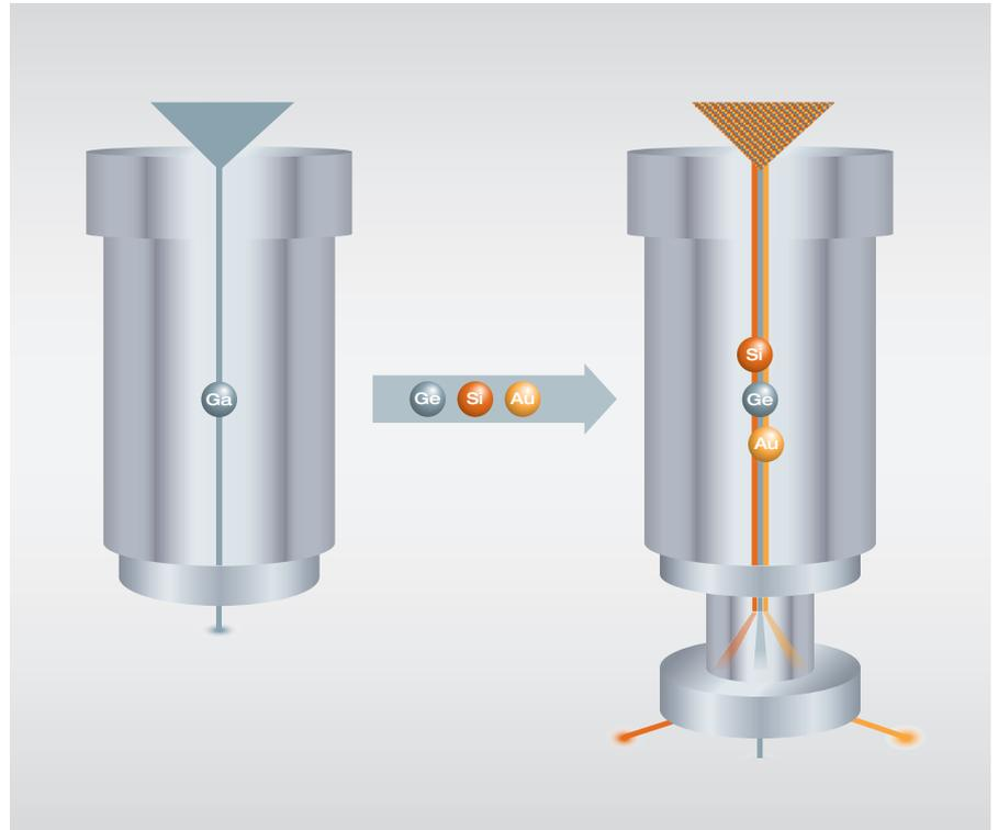
Figure 11: The extended nanoFIB with IONselect upgrade including alloy ion source and ion selector
