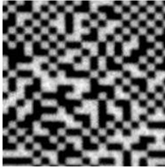
**Magnetic domains defined by specific low-dose ion beam damaging (intermixing of multi-layers) without creating any surface topography. Reproduced with permission from Gierak J, Mailly D, Hawkes P, *et al.* Exploration of the ultimate patterning potential achievable with high resolution focused ion beams. *Applied Physics A* 2005;80:187-94 © Springer**
