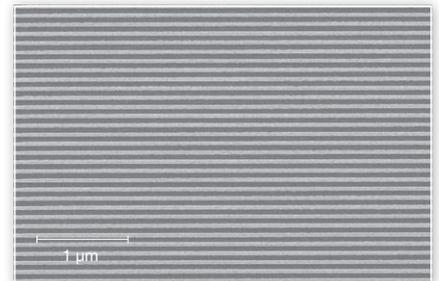
60 nm pitch grating in PMMA
