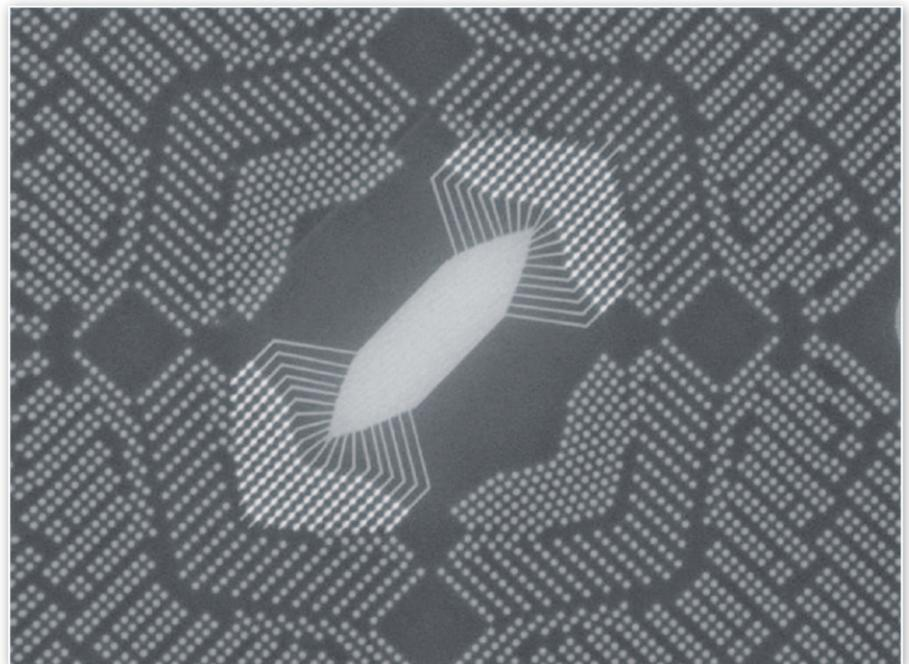
CMOS decoder circuit, aligned ebeam pattern with CMOS Metal 5 vias;
