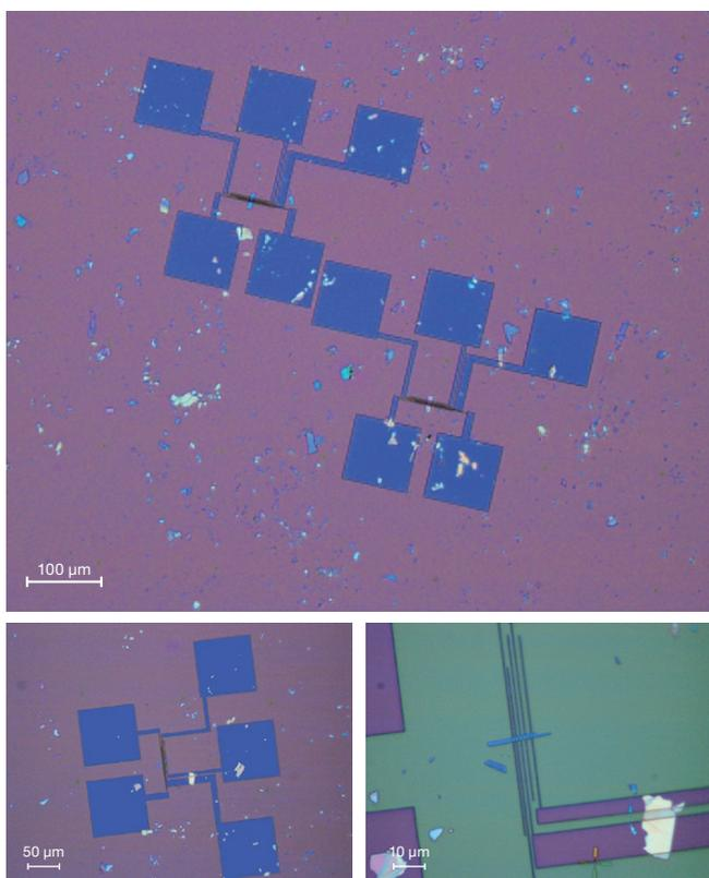
**Figure 4** Lift-off mask for electrodes defined by electron beam lithography with precise placement
