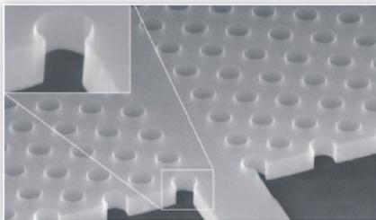
Advanced EBL: Photonic crystal structure in membrane;
