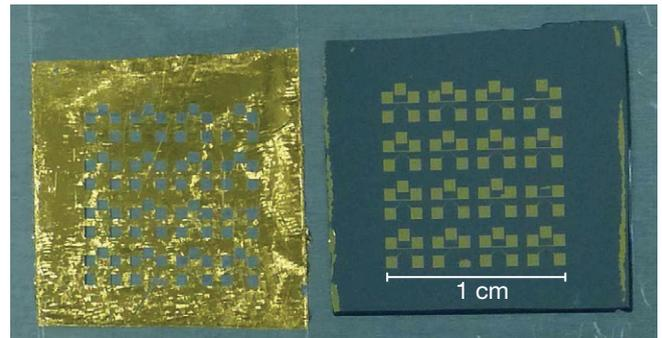
**Figure 9:** 1  $\text{cm}^2$  array of contact pad structures and the tape after peeling.
