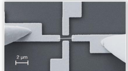
Freely suspended tungsten deposit between gold contacts, used for electrical conductivity measurement with nanoprobes.
