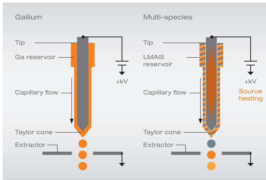
Figure 3: Schematics of Ga FIB ion emission (left) and schematics of LMAIS FIB including source heating (right)
