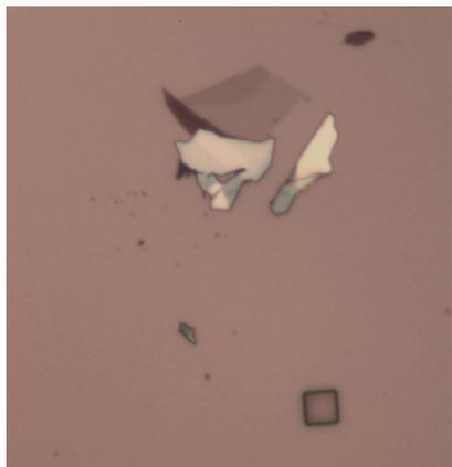
**Figure 6** Coarse optical localization of flakes
