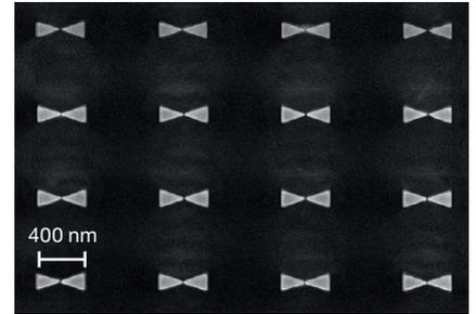
c) Li FIB adjustment of the gap size of the bowtie nanoantenna
