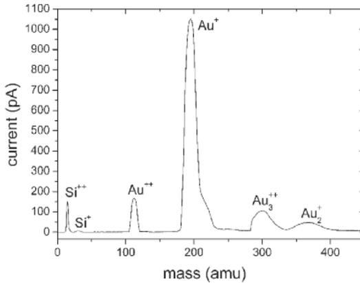
**Mass spectrum of a AuSi alloy ion source providing a range of different ion species. Image produced by Raith**
