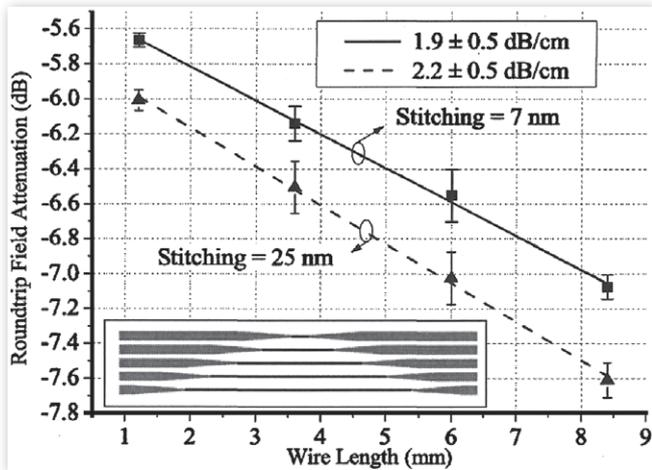
**Figure 6:** Propagation loss data for two sets of photonic wire waveguides that have different average stitching errors. The inset shows a sketch of the pattern used for the experiment. Adapted from [1]. Stitching errors increase the propagation loss dramatically.
