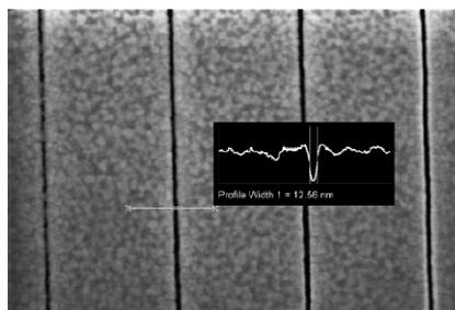
Figure 14: 13nm Si ion beam for Au layer
