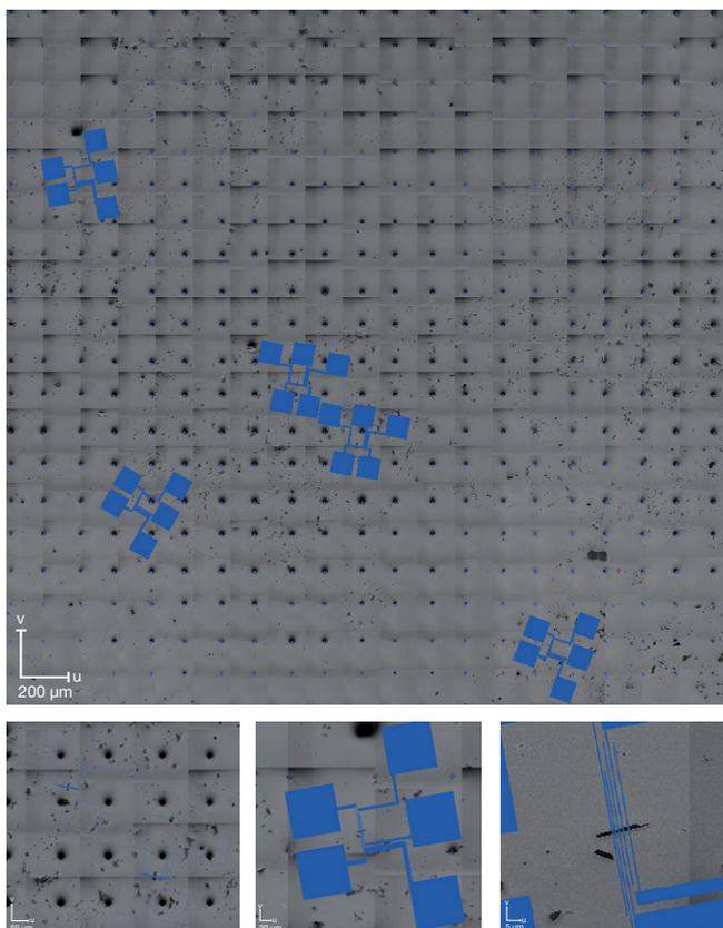
**Figure 3** Aligning electrode patterns onto large area SEM image to functionalize selected graphene flakes
