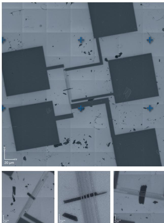
**Figure 5** Metalized electrodes functionalizing selected graphene flakes
