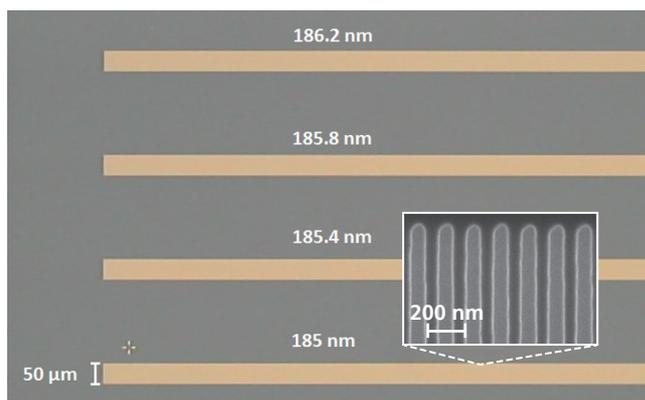
**Figure 5:** Optical microscope image (10x) of Bragg gratings with periods from 185 nm to 186.2 nm.
