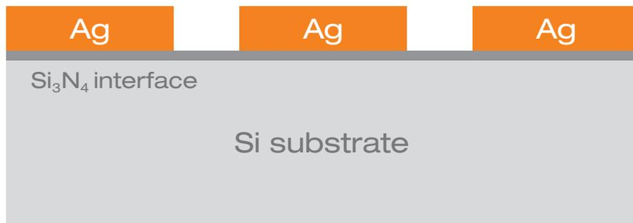
Figure 13: Illustration of the milling strategy on a functional film of a layered sample to avoid contamination
