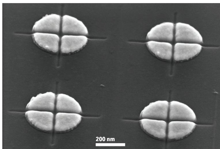
FIGURE 4 SEM micrographs of 40 nm thick segmented gold islands made by EBL plus precisely overlaid milling of crossing lines. Localized surface plasmons interact through the approximately 20 nm wide gaps that were intentionally overmilled deeper into the silicon, as this feature was predicted to favorably affect electromagnetic field enhancement<sup>[24]</sup>
