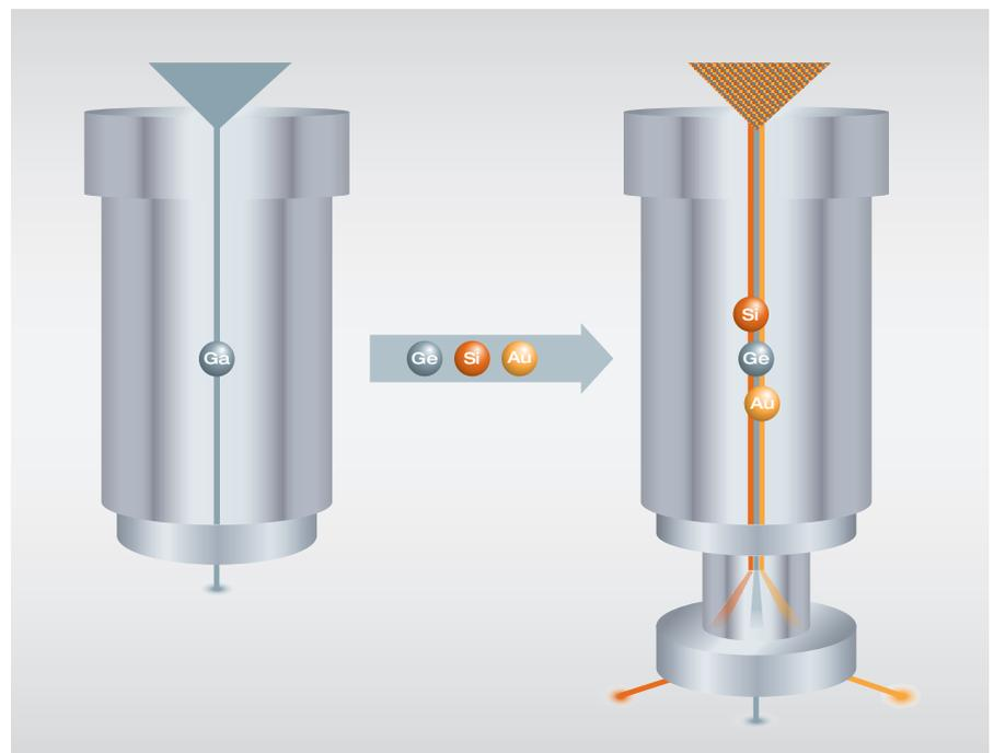
Figure 1: Schematics of nanoFIB column for Ga FIB (left) and nanoFIB with IONselect extension including LMAIS and Wien filter (right)
