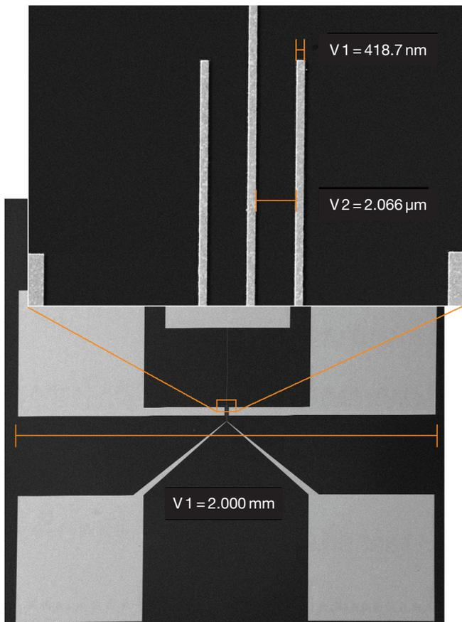
**Figure 8:** SEM images of a gold contact pad structure 2 mm in size, including 400 nm thick contact lines in the center.
