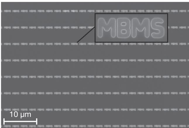
**Figure 1:** Modulated-Beam-Moving-Stage (MBMS) allows fabrication of any periodic structure without stitching.
