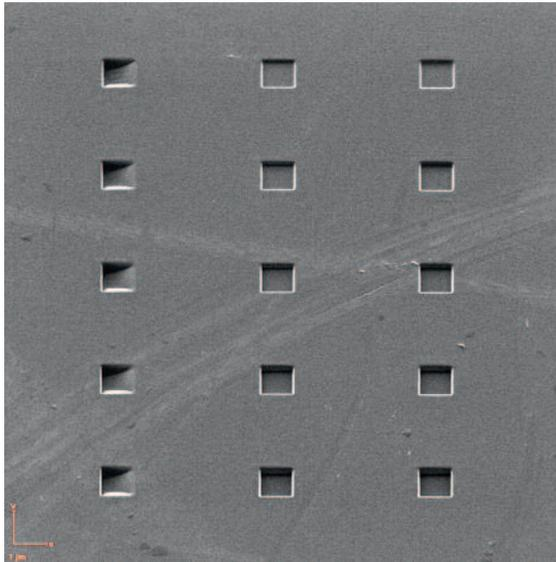
**Milling results for 1 $\mu$ m squares in SiC with constant dose per line, while the total dose is applied in 1 (left) or 1000 loops (right). The scan strategy consists of lines in Y direction from right to left on all boxes and shows pronounced redeposition and edge effects in case of the single loop approach. Image produced by Raith**
