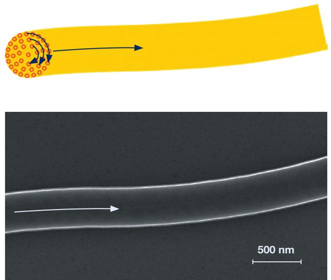
**Figure 5:** A 500nm wide path exposed in FBMS mode with uniform dose distribution in 200nm thick HSQ. The orange dots in the FBMS area sketch represent repetitively applied lateral beam deflection. G. Piaszenski, Raith GmbH.
