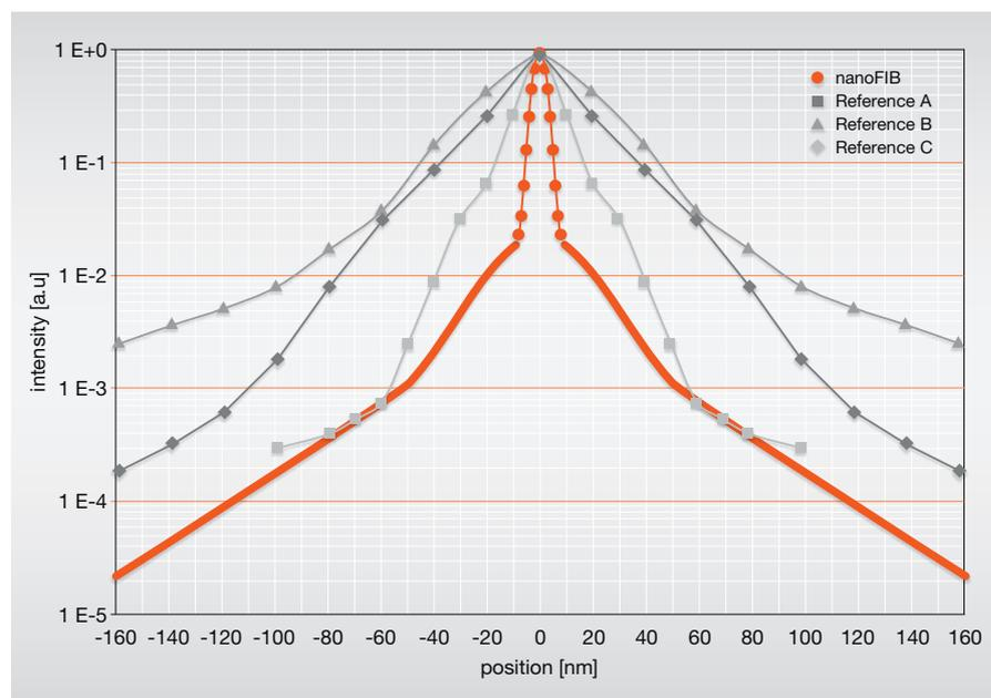
Figure 5: Beam current distribution for nanoFIB showing a narrow and large central spot and low tails compared to different data of conventional FIB technology. Reference results A to C can be found in 3, 4, 5, respectively
