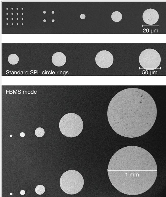
**Figure 6:** SEM images of gold circles with varying sizes. Circles over 50 μm were milled using FBMS (fixed-beam moving-stage) mode.
