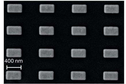
b) Step 2: Li FIB for fine shaping of rectangular boxes to fabricate bowtie structures at highest resolution
