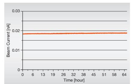
Figure 1: Probe current of Raith's nanoFIB™ Ga focused ion beam showing excellent long-term stability
