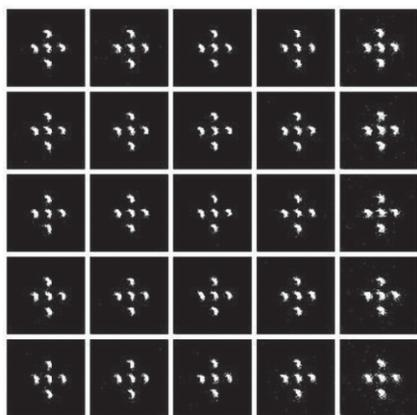
Figure 3: Features are placed free of stigmatism and distortions, accurately, and all over a single write field after corrections to enable write-field stitching for nanofabrication
