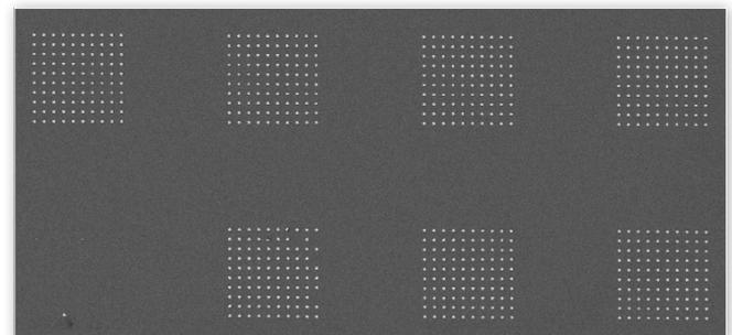
**Figure 2:** Test arrays of 800 nm circles after peeling, created with Au<sup>++</sup> ions at different line doses (increasing dose from lower left to upper right array).
