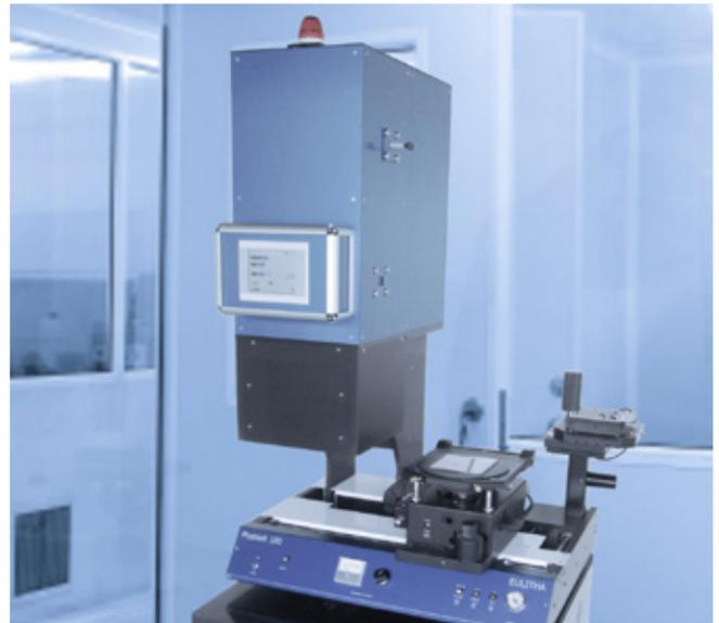
Figure 4: PhableR 100 Displacement Talbot Lithography System
