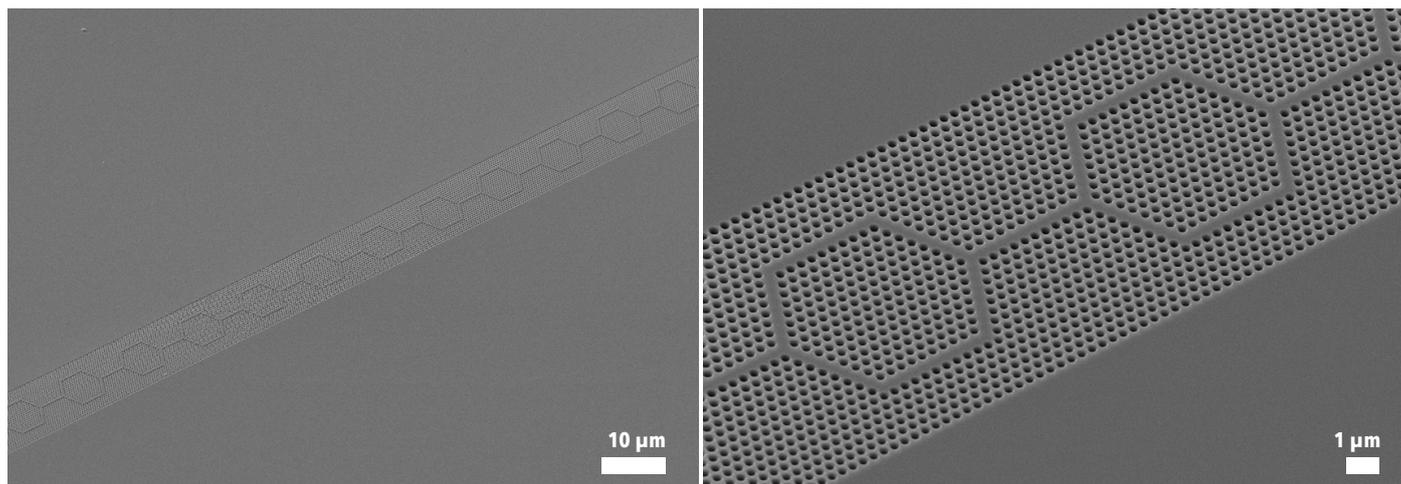
**FIGURE 5** Photonic waveguide structure prepared using a Ga FIB and precision stage technology for write field stitching
