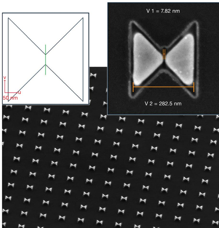
Another example of a plasmonic array is shown in figure 5. Here a 25 μm x 25 μm array of 625 gold nano-disks has been created by sketch & peel, including sinusoidal low-dose cuts inside the disks. This pattern could be milled within a mere 25 min at 1.7 pA Ga<sup>+</sup> beam current.
