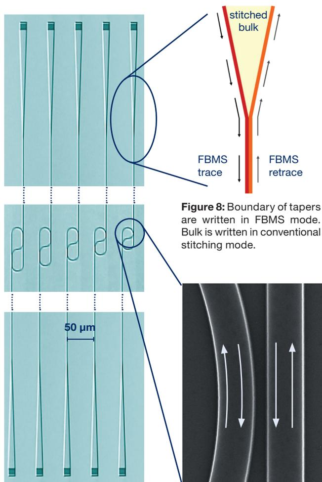
**Figure 8:** Boundary of tapers are written in FBMS mode. Bulk is written in conventional stitching mode.
