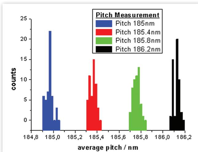
**Figure 6:** Pitch variation within Bragg gratings. The pitch was measured as an average of distance measurements between 100 lines.
