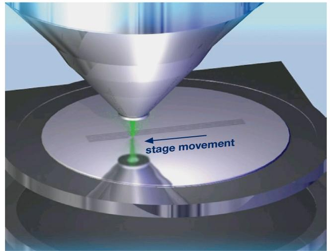
**Figure 3:** New Fixed-Beam-Moving-Stage mode enables patterning of endless paths with virtually no stitching errors: The beam is fixed while the stage is moving.
