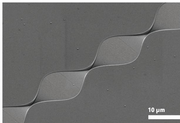
FIGURE 3 Gallium FIB has been used to fabricate a micro-fluidic mixing channel by direct 3D structuring (lateral pattern definition plus dose variation) over a total length of 1 mm<sup>[22]</sup>
