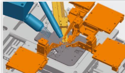
CAD view inside the eLINE Plus vacuum chamber showing the compact geometry with integrated GIS, SE- and EDX-detector and 4 nanomanipulators. Anti-collision control software features prevent system damage.
