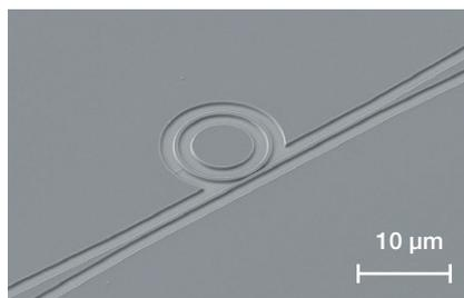
Figure 7: 4 mm waveguide and coupler directly milled with Ga ion beam into silicon substrate by nanoFIB
