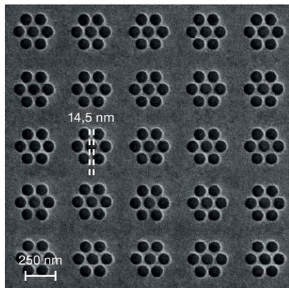
Figure 10: Li FIB patterning of HNH in 50 nm Au substrate and subsequent Li ion beam imaging
