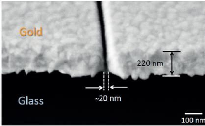
Figure 9: SEM image of a 45-degree-tilted 20 nm groove in 220 nm Au film on glass substrate<sup>17</sup>
