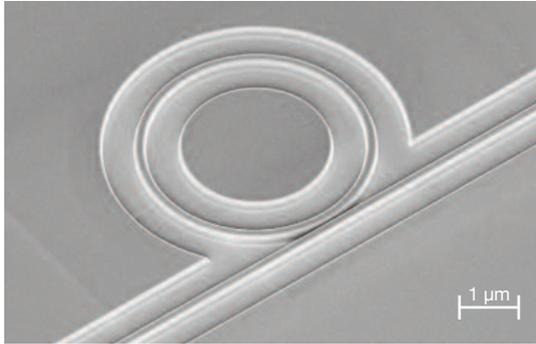
**Photonic device (wavelength and coupler) in a silicon substrate created by direct milling with a focused gallium ion beam. Image produced by Raith for Professor Peng, Peking University, China**
