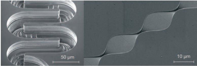
Microfluidic mixer structures can be fabricated by 3D FIB machining both on a large micrometer scale (left, compare Ocola *et al*, 2013) as well on a micrometer/submicrometer scale (right, compare Palacios *et al* 2010) by complex and precise patterning control in combination with sophisticated sample positioning. Reprinted with permission from Ocola LE, Palacios E. Advances in ion beam micromachining for complex 3D microfluidics. *J Vac Sci Technol* 2013;31:06F401
