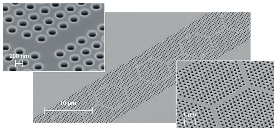
Figure 8: Structure of photonic elements directly milled into Si bulk material. Lowest beam tails result in straight cylinders with 200nm diameter and 200nm depth. In particular, edges are fabricated sharply and are not rounded or affected by beam tails
