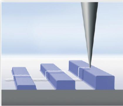
Operation principle of NanoSense distance sensor option
