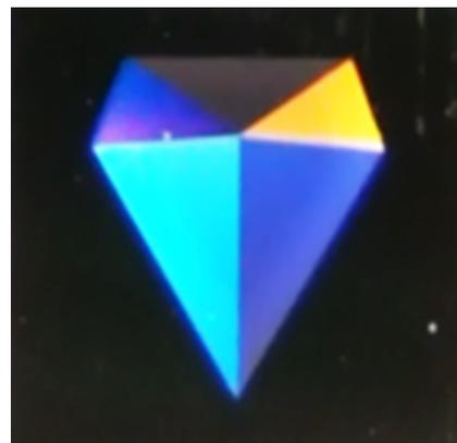
Figure 5: Photograph of the complete pattern after etching. Colors represent the different grating orientations. [1]
