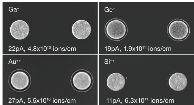
**Figure 3:** 800 nm circles created with 4 different ion species and corresponding optimum line doses for successful sketch & peel.
