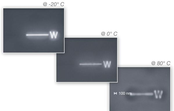
Tungsten deposit under identical deposition parameters but different temperatures
