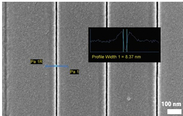
FIGURE 1 FIB line cuts in a 20 nm thick chrome layer (SEM image) showing the patterning fidelity of Ga focused ion beam
