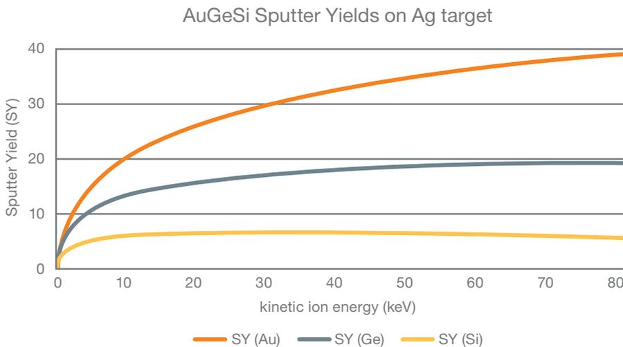
Figure 12: AuGeSi sputter yield as a function of ion energy
