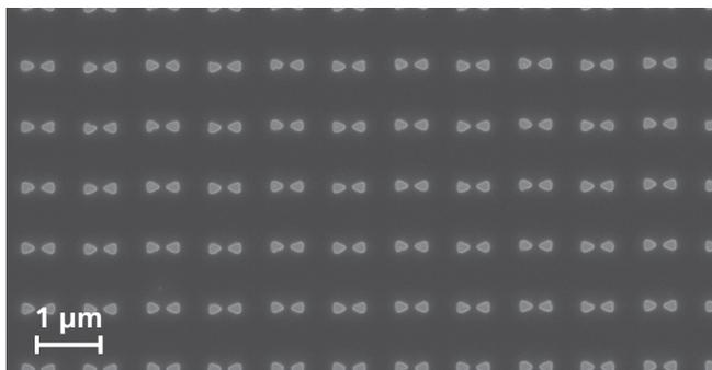
**Figure 11:** Array of bowtie structures for nanoantennas.
