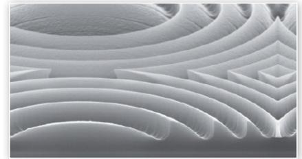
Fresnel lens array in 5 μm thick resist
