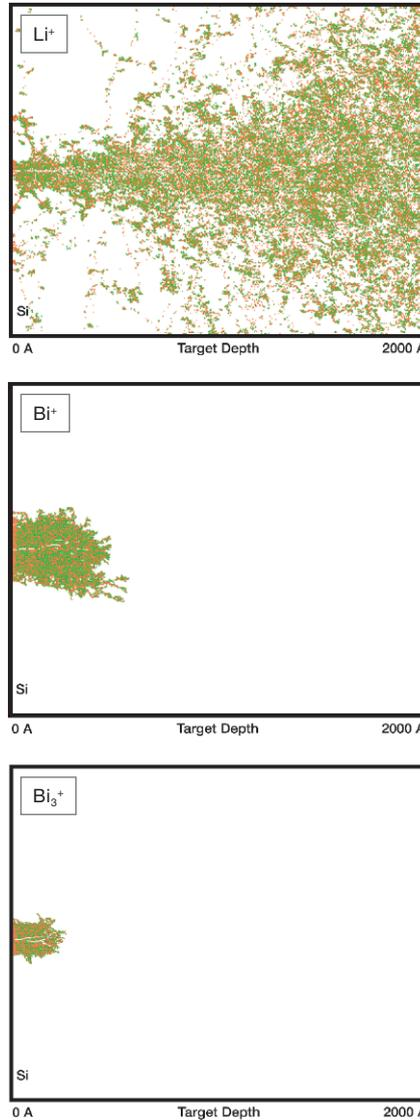
Figure 9: TRIM acceleration voltage 35 kV, target Si substrate
