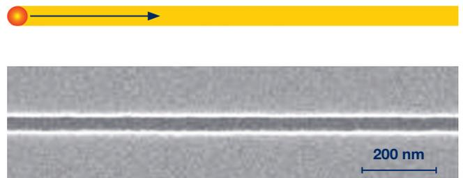
**Figure 4:** A perfectly straight FBMS line of about 13mm length etched in Si. The orange dot represents a fixed beam in high resolution mode. Courtesy of H. Neubauer et al., University of Göttingen, Germany.
