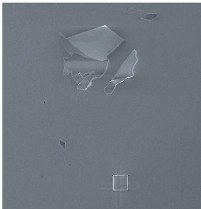
**Figure 7:** Fine SEM-based localization of flakes
