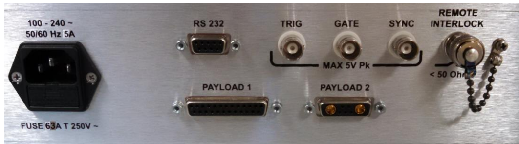
Figure 17 Power Supply Connections (Payload2 not installed)
