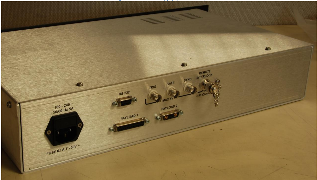
Figure 12 Power Supply (Connections)
