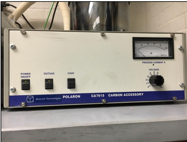
Figure 2.4: The control panel for the CA7625
