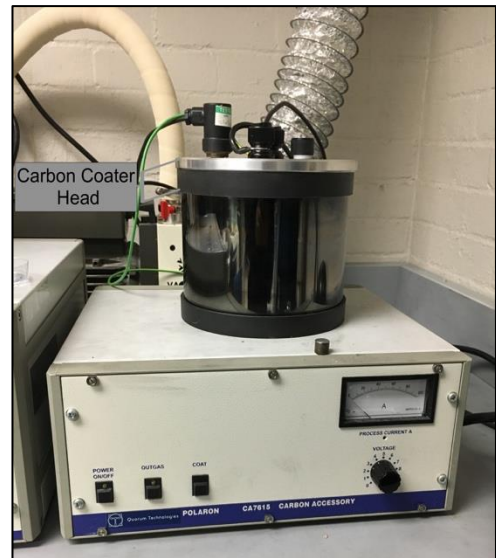
Figure 2.5: The CA7625 control panel with its head
