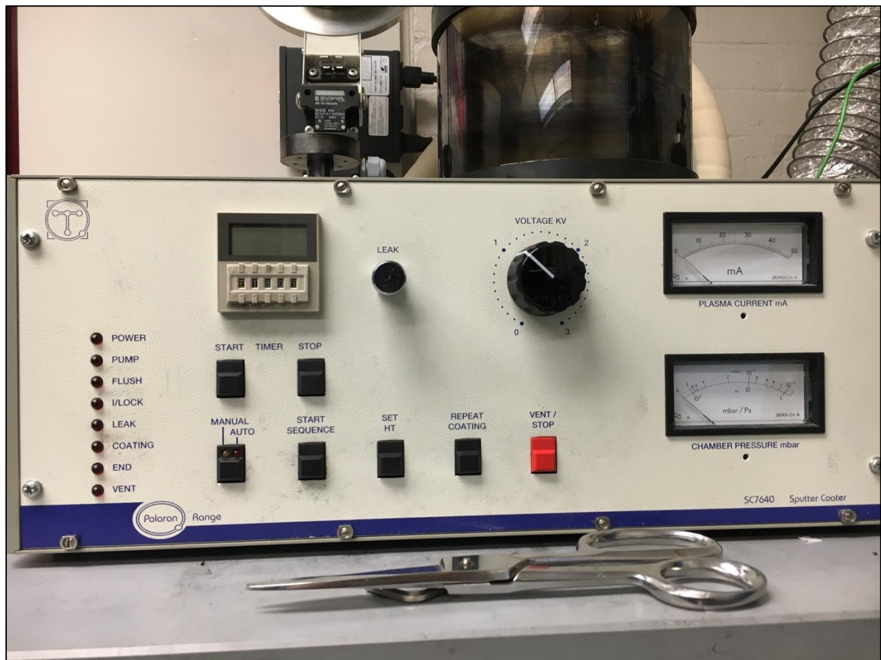
Figure 2.3: The control panel for operating the SC76400
