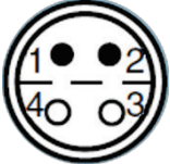
Figure 5: Sensor connector, LEMO FFA.0S.304.CLAC32, front view
