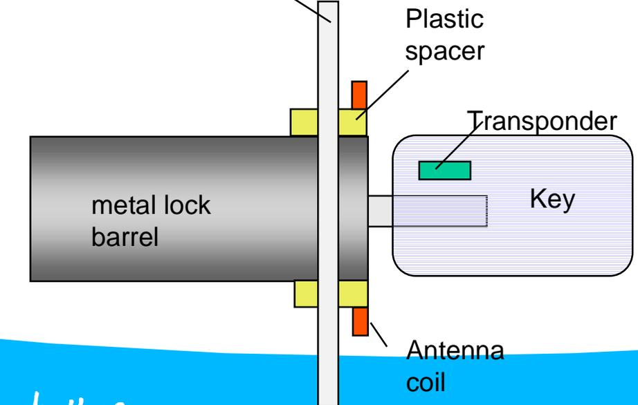
The upper design example normally results in higher coupling factors
