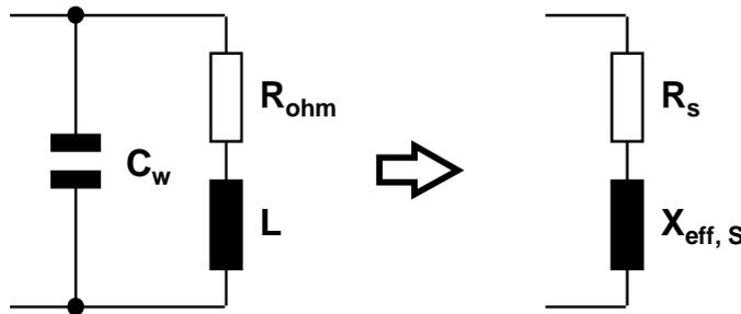
$$R_s = \frac{R_{ohm} \cdot \frac{L}{C_w} - \frac{R_{ohm}}{\omega \cdot C_w} \cdot \left( \omega \cdot L - \frac{1}{\omega \cdot C_w} \right)}{R_{ohm}^2 + \left( \omega \cdot L - \frac{1}{\omega \cdot C_w} \right)^2} \quad Q_L = \frac{X_{eff,S}}{R_s}$$
