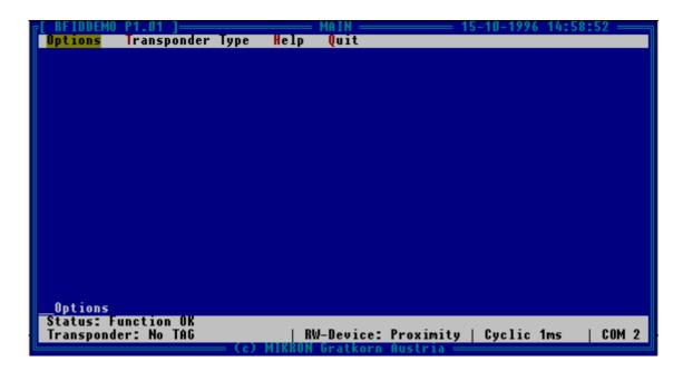
The two bottom lines display error messages, information about transponder, interface and read/write device.
