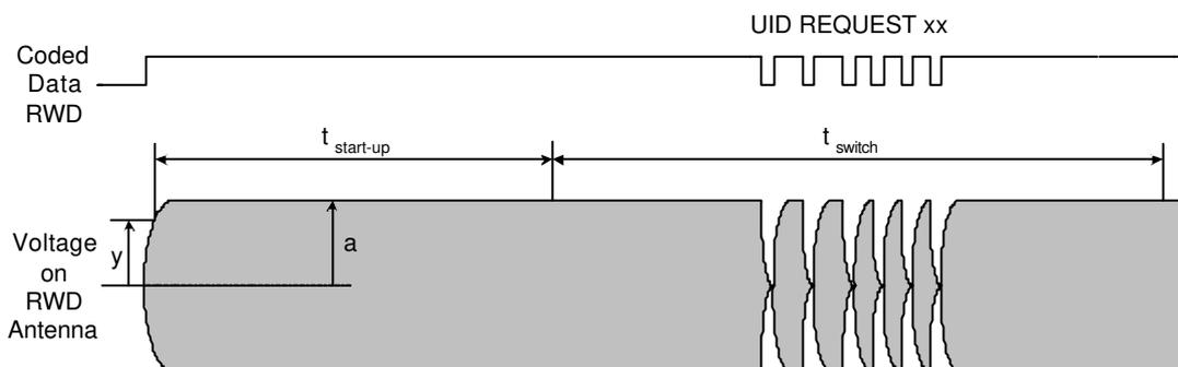
Within the time  $t_{switch}$  a HITAG S Transponder configured in TTF Mode can be switched into RTF Mode by a UID REQUEST xx command. The HITAG S Transponder responds to this command with the UID and changes into Init State .
