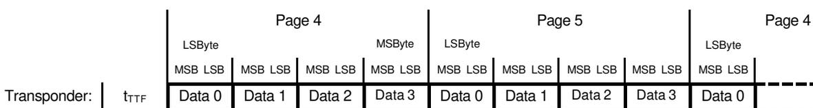
The data rate and the data coding can be chosen independently by configuration Bits TTFC, TTFDR 0 and TTFDR 1.
