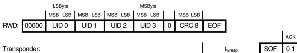
The 'start of frame' (SOF) pattern and the acknowledge (ACK) is transmitted in Manchester Coding.
