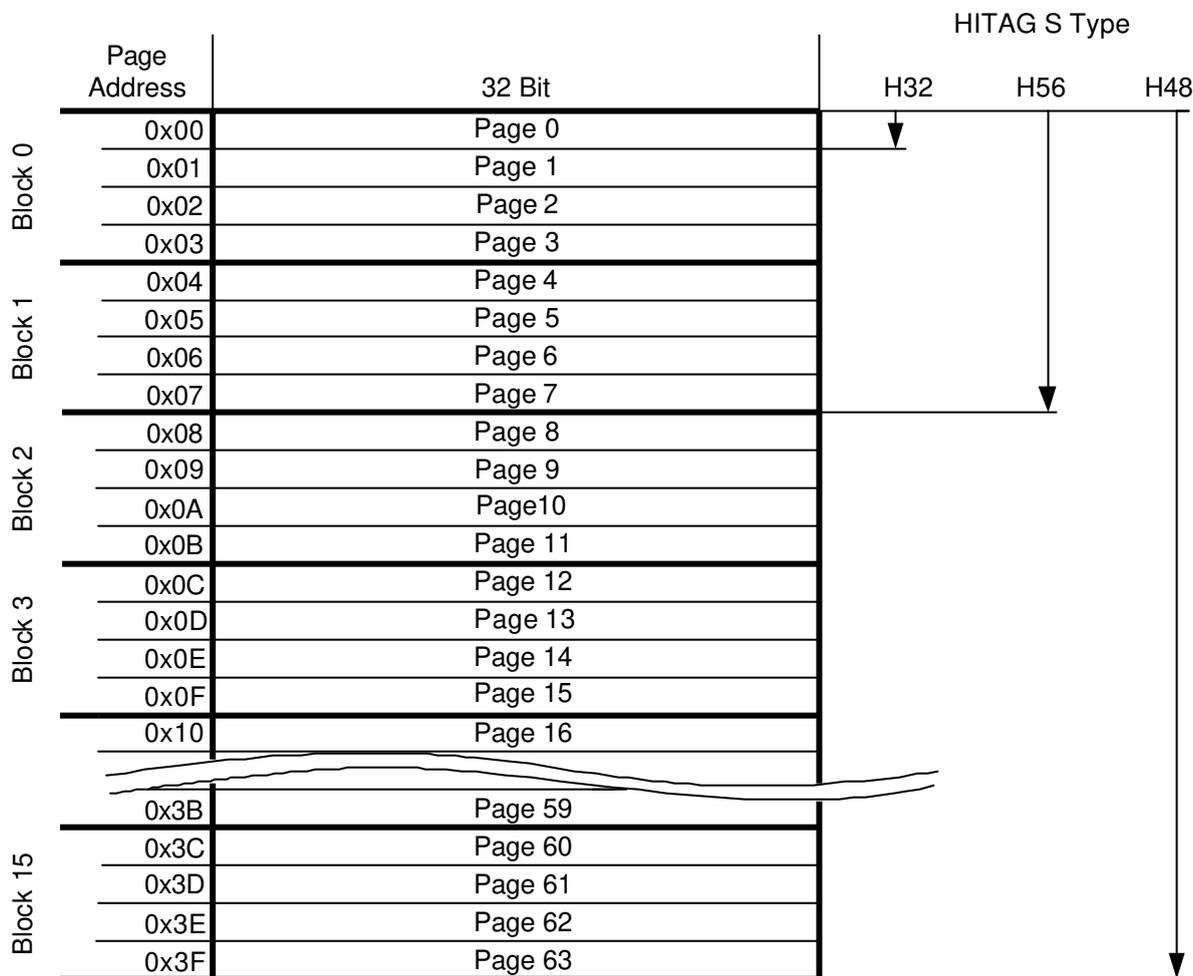
The EEPROM has a memory capacity up to 2048 Bit and is organised in 16 Blocks consisting of 4 Pages each for commands with Block access. A Page consists of 4 Bytes each (1 Page = 32 Bits) and is the smallest access unit.
