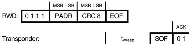
After the response wait time  $t_{wresp}$  the HITAG S Transponder responds with a SOF and an acknowledge to confirm entering the Quiet State.
