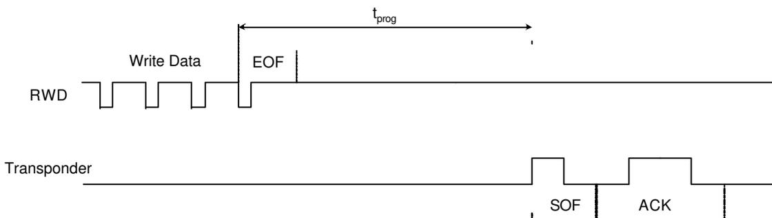
When receiving the EOF of the write data from the Read/Write Device, the transponder waits  $t_{prog}$  before transmitting the SOF and acknowledge to confirm correct programming.
