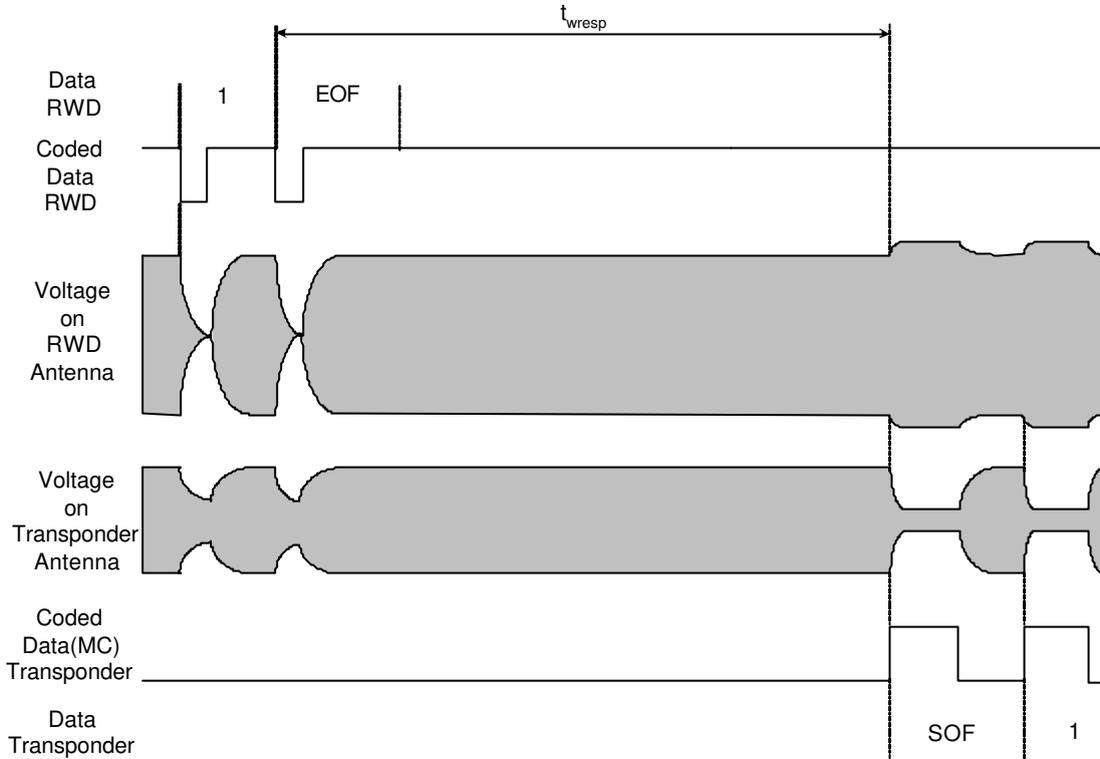
When receiving a End of Frame (EOF) condition from the Read/Write Device, the transponder waits  $t_{wresp}$  before transmitting data.
