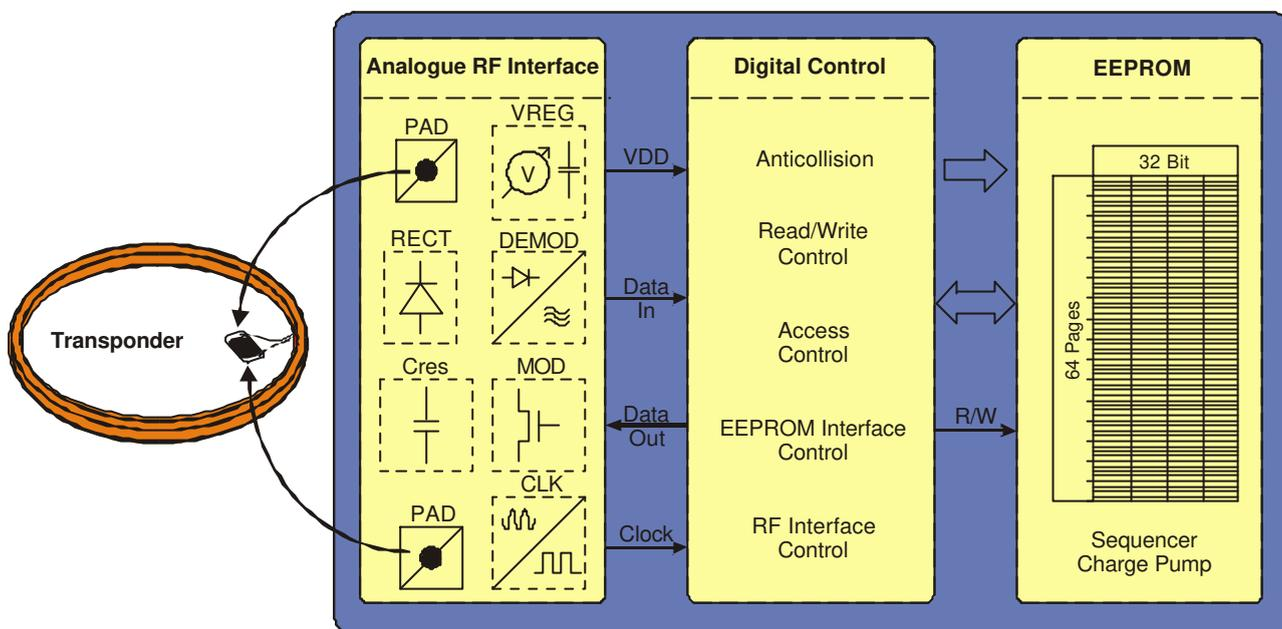
The HITAG S Transponder requires no internal power supply. The contactless interface generates the power supply and the system clock via the resonant circuitry by inductive coupling to the Read/Write Device (RWD). The interface also demodulates data that are transmitted from the RWD to the HITAG S Transponder, and modulates the magnetic field for data transmission from the HITAG S Transponder to the RWD.
