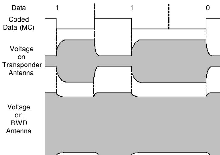
The modulation ratio of the RWD antenna voltage depends on the coupling factor of the antenna configuration (RWD antenna size, transponder antenna size, distance between the antennas,...).
