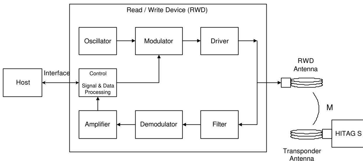
A control and data processing unit controls the modulation of the carrier signal and processes data coming back from the demodulator circuit.
