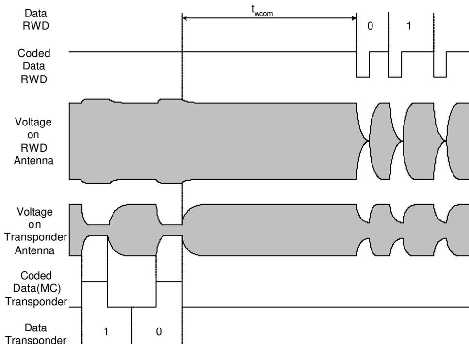
When the Read/Write Device has received the response from the HITAG S Transponder to a previous command, the RWD has to wait a time  $t_{wcom}$  before sending a subsequent command or Write data after a Write command.
