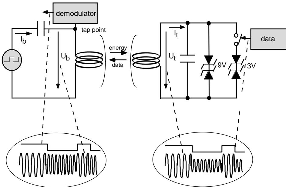
Fig.10 Data transfer from transponder to basestation
