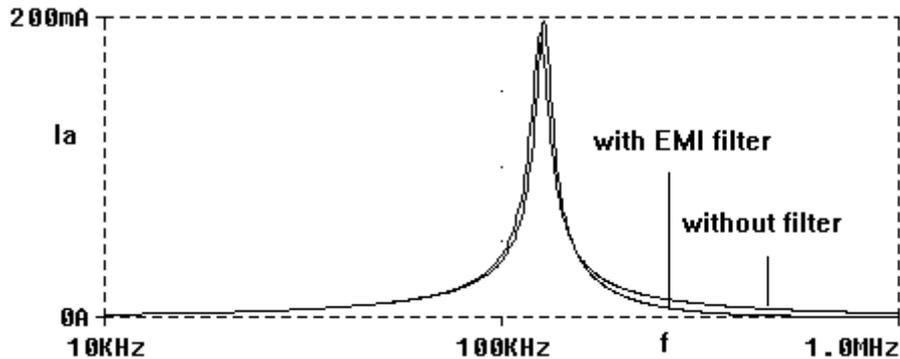
There are other filtering solutions possible too. In case of higher order passive filters, care should be taken of the losses in the filter elements at resonance frequency.
