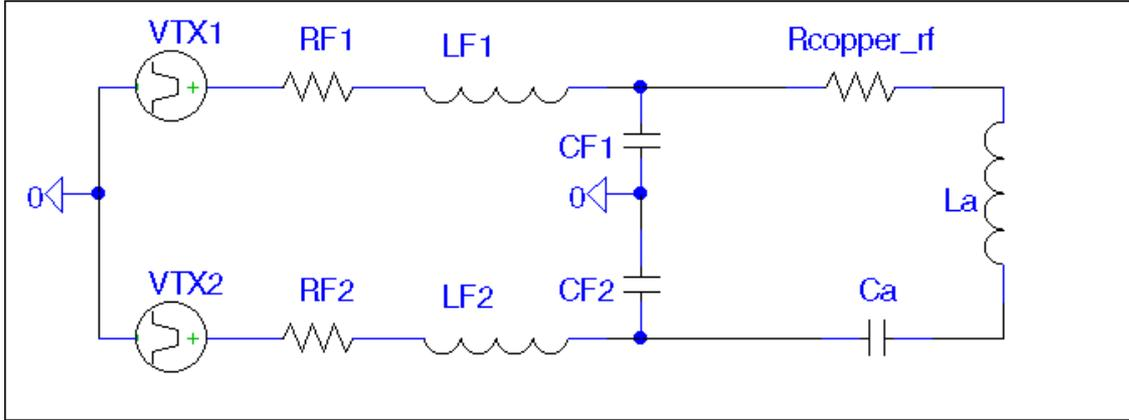
The filter is built of  $R_F$ ,  $L_F$  and  $C_F$ . Every element is split into two parts to design a symmetric filter with respect to ground. This is done to filter the voltage at the TAP-point with respect to both driver outputs.
