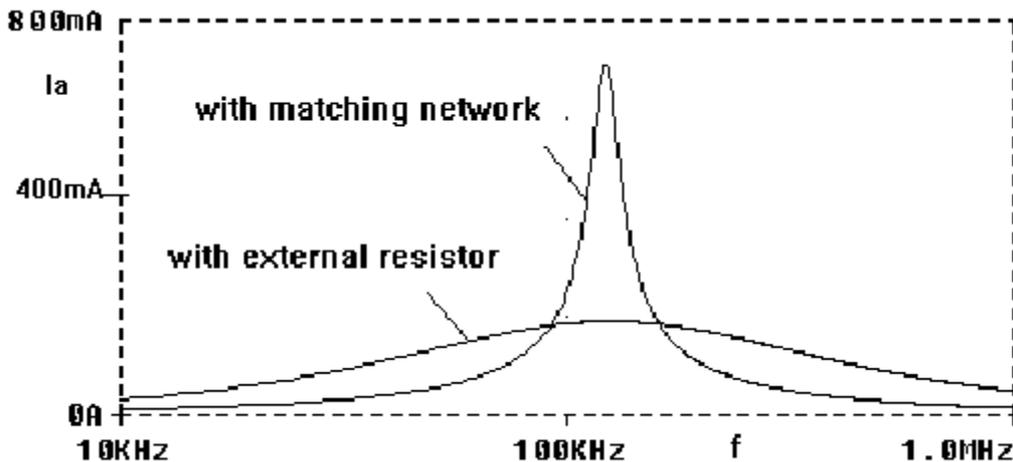
It can be seen, how the external resistor decreases the quality factor of antenna, whereas the matching network has no influence on the quality factor. Thus, the maximal transmission range of antenna can be achieved.
