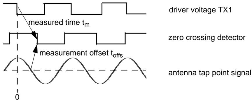
Fig.21 Phase measurement
