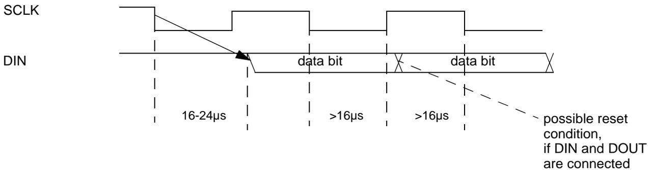
Fig.4 Data transfer from the HTRC110 to the µC with glitch filters on
