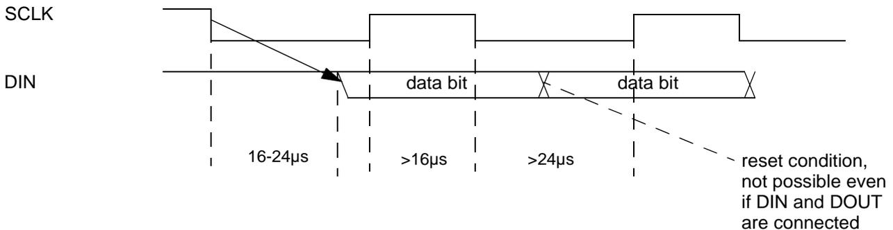
Fig.5 Data transfer from the HTRC110 to the µC with glitch filters on
