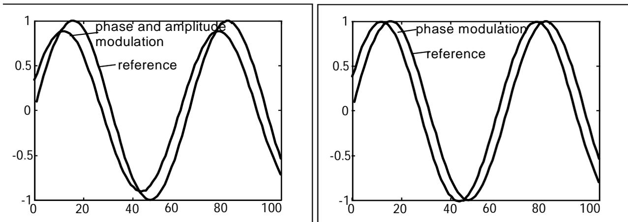
Fig.13 Mixture of amplitude and phase modulation / pure phase modulation
