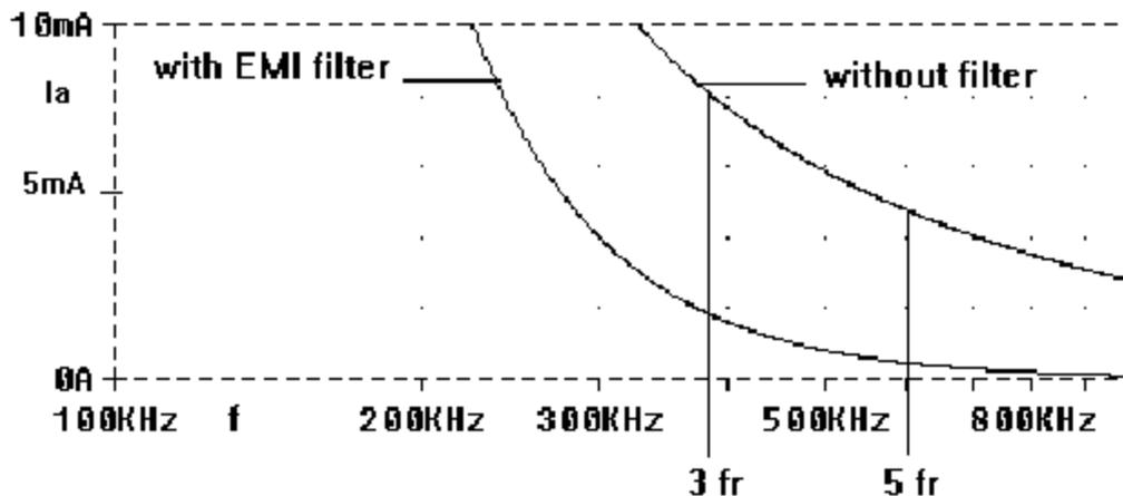
Another advantage of the proposed filter is, that the resonance frequency of the antenna is almost not influenced, however the antenna should be tuned including the filter as described in this application note. When using an EMI filter, the offset compensation constant should be readjusted (see chapter 9.2.4).
