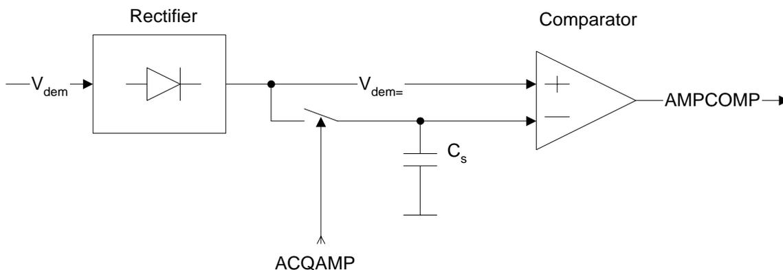
When the *ACQAMP* control bit is set by a *SET\_CONFIG\_PAGE* command, the actual demodulator signal amplitude  $V_{\text{dem=}}$  is stored in the capacitor  $C_s$ . After resetting the *ACQAMP* bit, the status bit *AMPCOMP* is set, when the actual signal amplitude is larger than the stored reference otherwise it is cleared.
