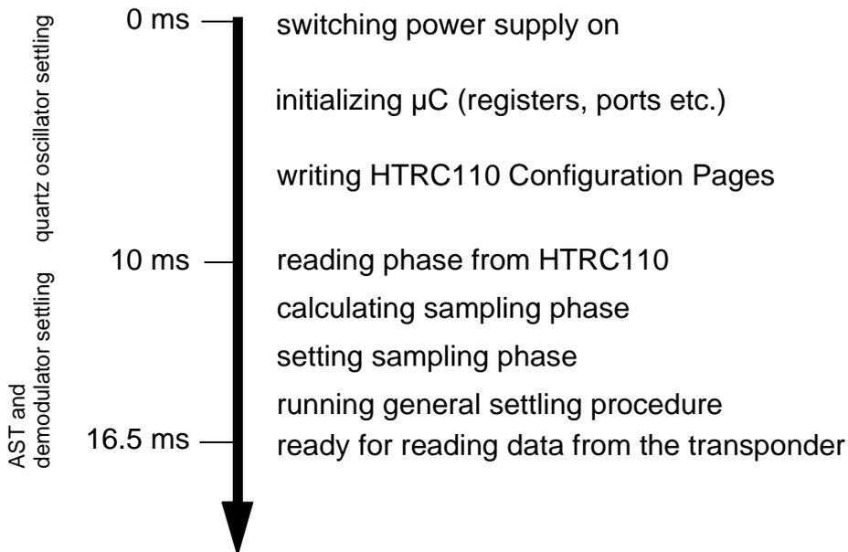
Fig.24 Example power-on sequence
