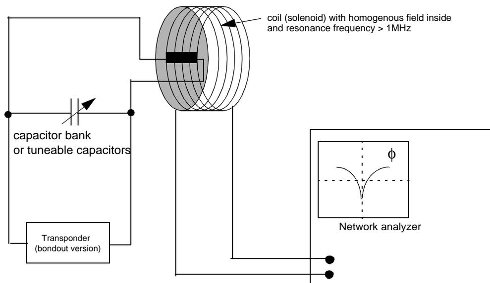
Fig.27 Contactless transponder resonance frequency measuring setup
