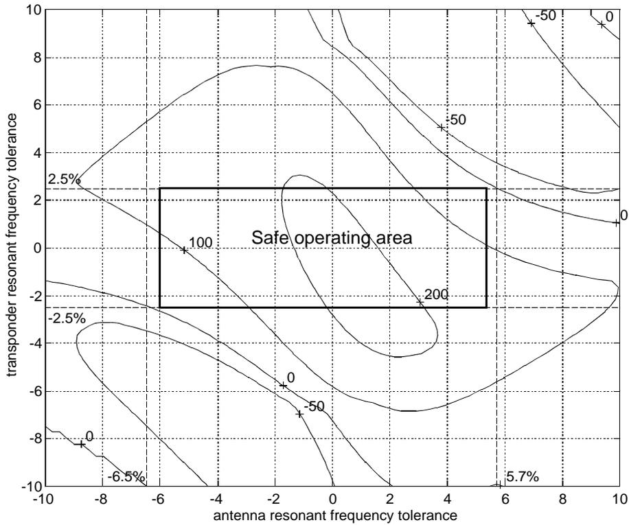
Fig.14 Example tolerance field of envelope demodulator
