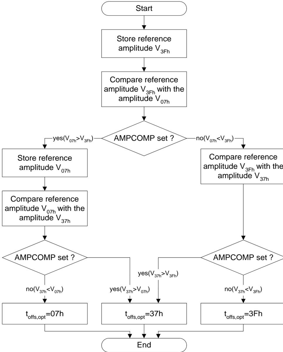
The voltage  $V_{xyh}$  denotes the measured demodulator voltage using a compensation constant of  $xyh$ . At the end of this algorithm, the optimized compensation constant  $t_{offs,opt}$  is found. The number of compensation constants should be chosen in order to get a good compromise between computation speed and maximum deviation from the optimum compensation constant (e.g.  $n = 5, 7, \dots$ ).
