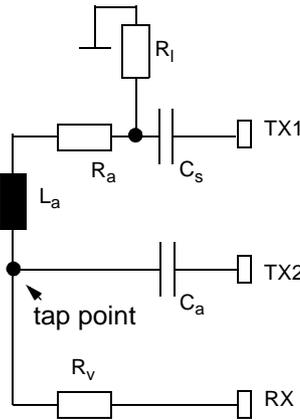
Fig.7 Antenna circuitry with driver protection
