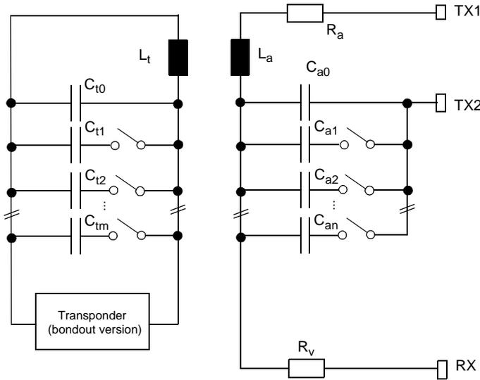
Fig.25 Tolerance field measurement circuit
