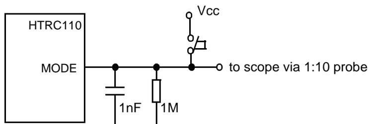
Fig.22 External circuitry for analog signal monitoring and unlocking test-mode prohibition
