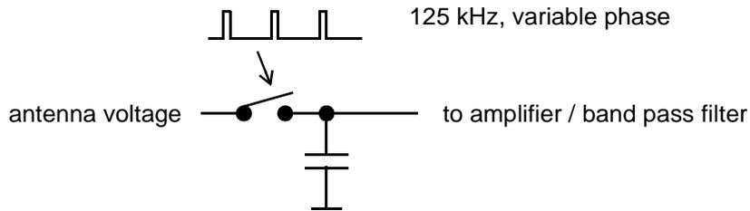
Fig.15 Sampling demodulator
