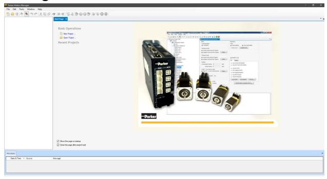
When first starting PMM, the Start screen will appear. A new project can be initiated or an existing project can be opened. As projects are created, they will appear under Recent Projects. The Start screen can be disabled or reenabled under Tools → Options. That menu also allows clearing the list of Recent Projects.
