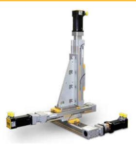
In the system shown above, the two subsystems would be attached to different masters, like Master 0 and Master 1. This would allow the controller to tightly coordinate moves within each subsystem, but would also allow each subsystem to maintain its independence from the other.
