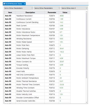
NOTE: Not all parameters are used in all products. For example, the ACR7xC controller does not have integrated steppers and thus the stepper drive parameters would all be 0.
