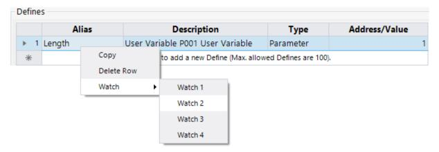
Bits and parameters can also be added to a watch window from the Motion Status Panel or Drive Status Panel. To add a bit or parameter, right-click on the indicator of interest and select a watch window:
