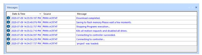
Informational messages appear in blue, warnings appear in yellow and errors appear in red. The Messages Window is particularly useful when troubleshooting connection issues with the controller. Notice the two warnings shown at the top of the image below:
