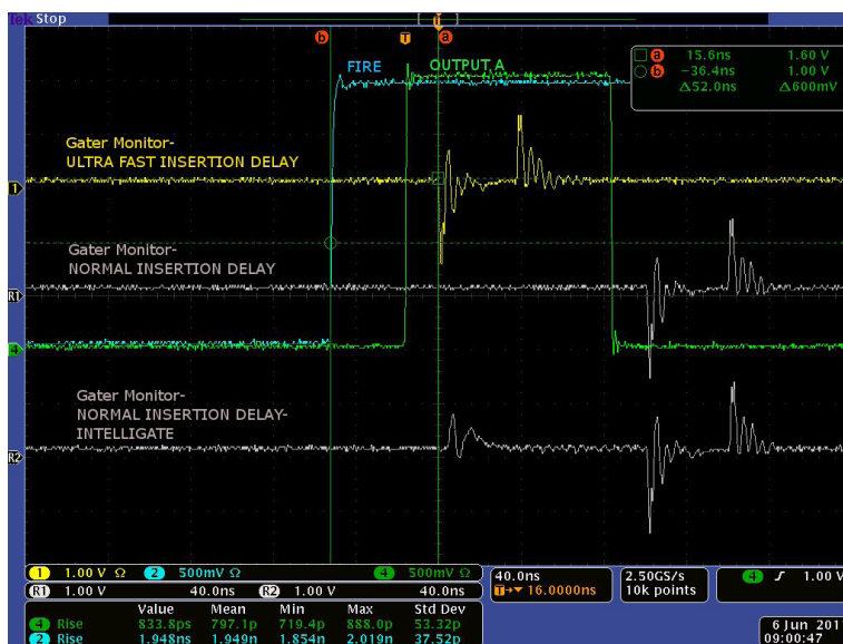
Fire pulse to intensifier opening using DDG
