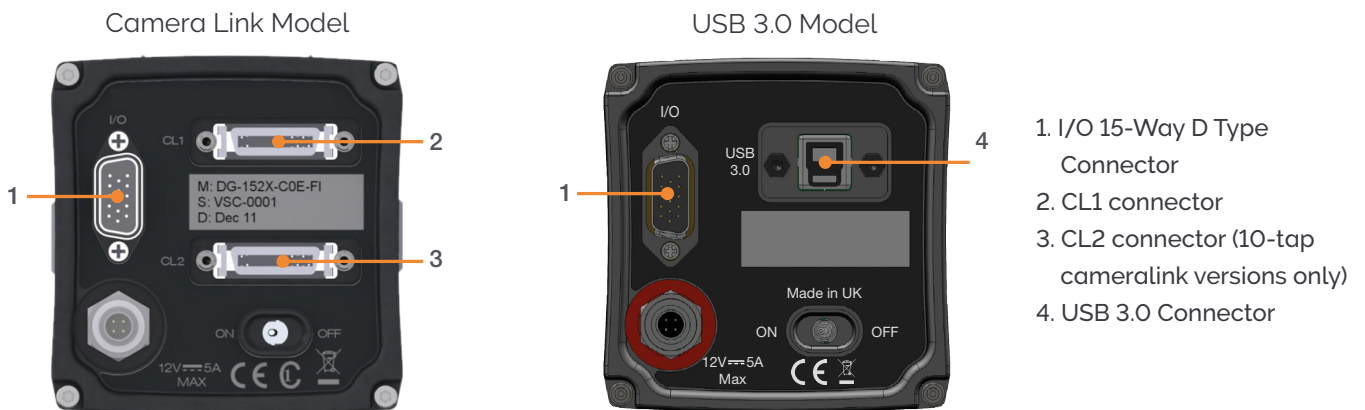
Figure 38: Connect the Zyla to the port on the PC by the connections shown above (Left) Camera Link model, (Right) USB 3.0 model
