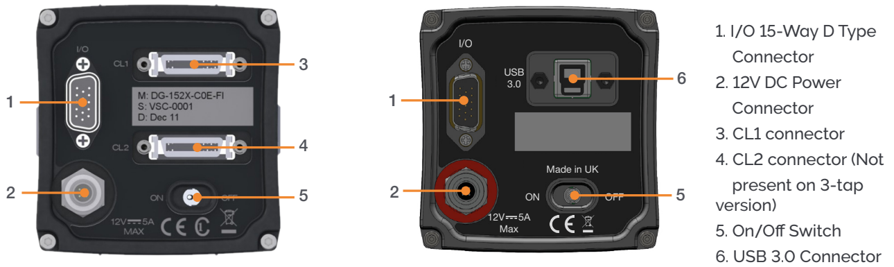
Figure 3: Zyla Back Plate Connections (Left) Cameralink versions (Right) USB 3.0 version
