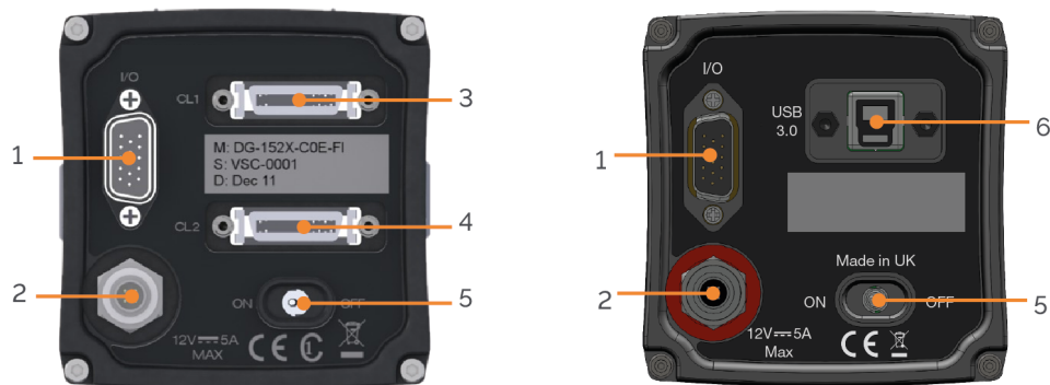
Figure 3: Zyla Back Plate Connections (Left) Cameralink versions (Right) USB 3.0 version
