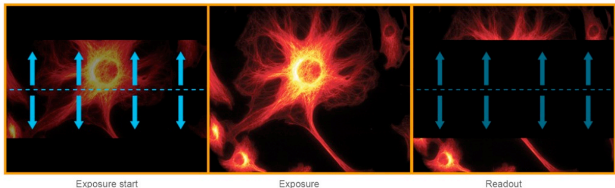
Figure 15: Rolling Shutter Exposure and Readout
