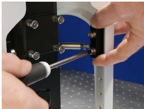
Figure 25 Adjust the position of the locator blocks
