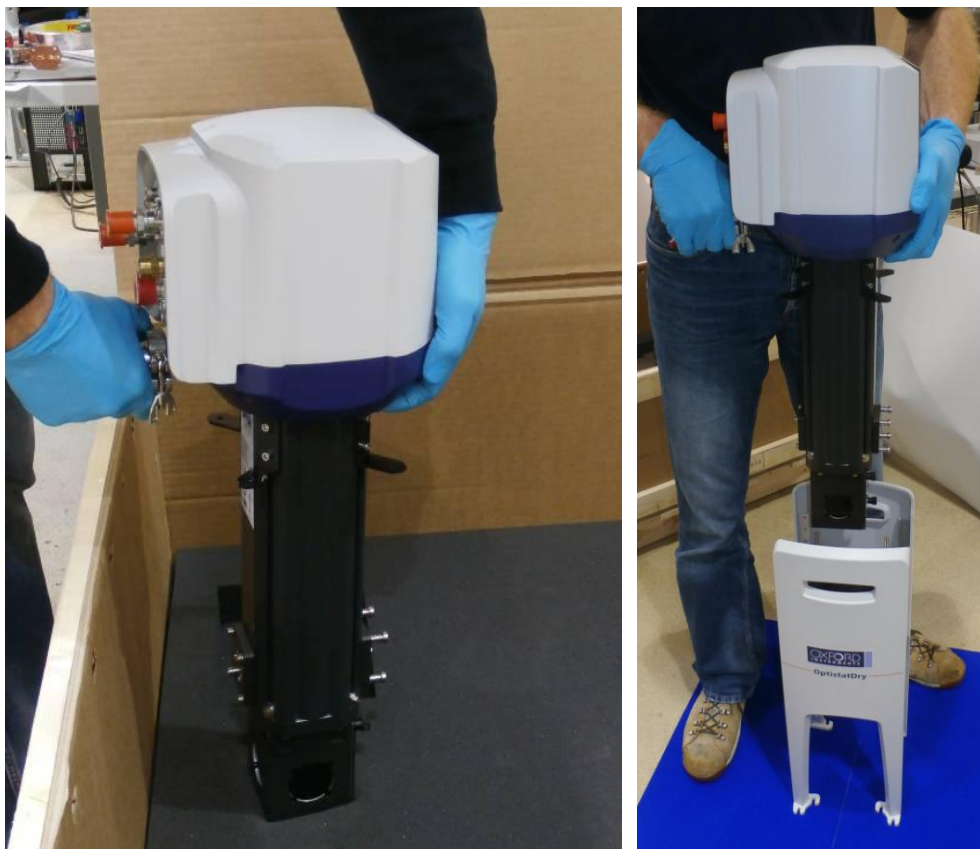
Figure 15 Lower the cryostat into the side panel assembly
