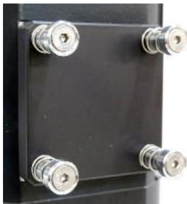
Figure 1 OptistatDry BL4 pressure relief plate
