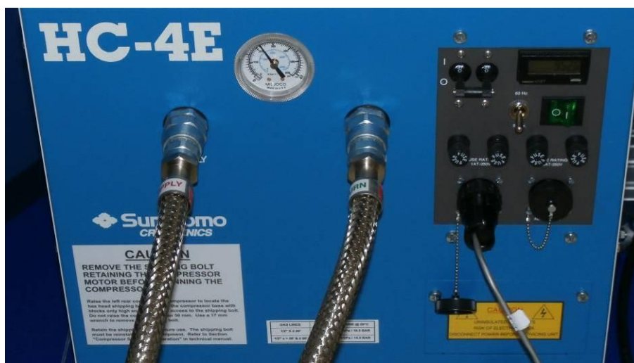
Figure 33 Make the helium line connections to the compressor
