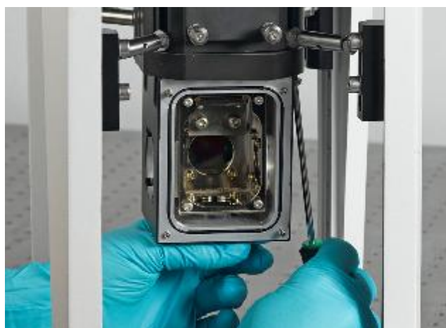
Figure 47 Remove Torx bolts in OVC body
