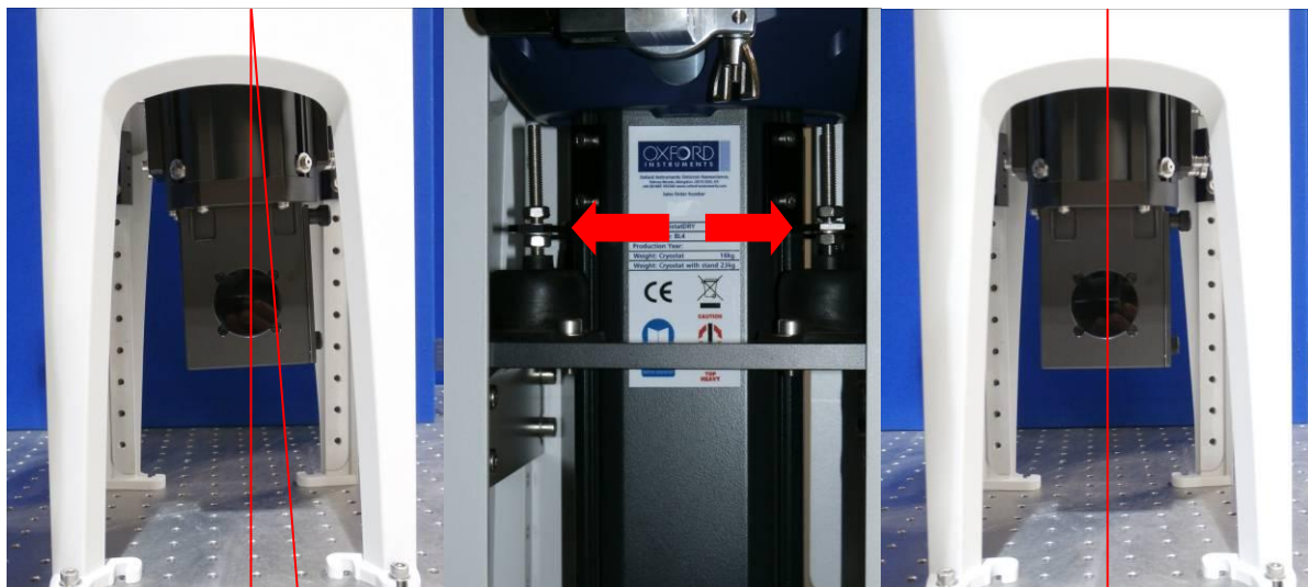
Figure 19 Adjust the vertical alignment of the cryostat
