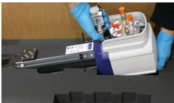
Figure 13 OptistatDry BL4 cryostat removal from packaging
