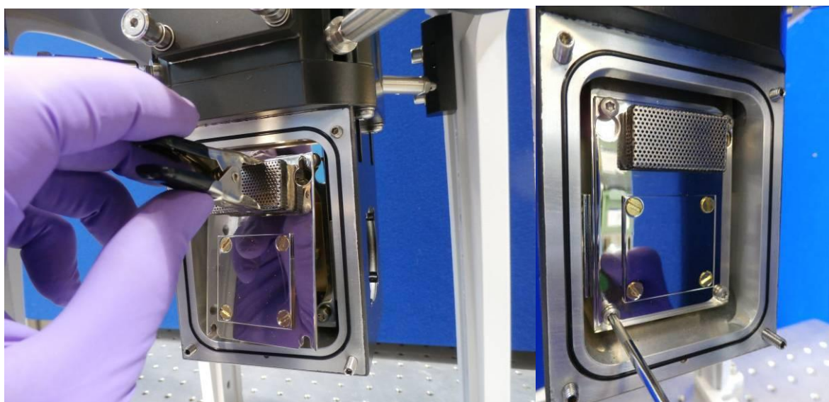
Figure 39 Replace radiation shield plate
