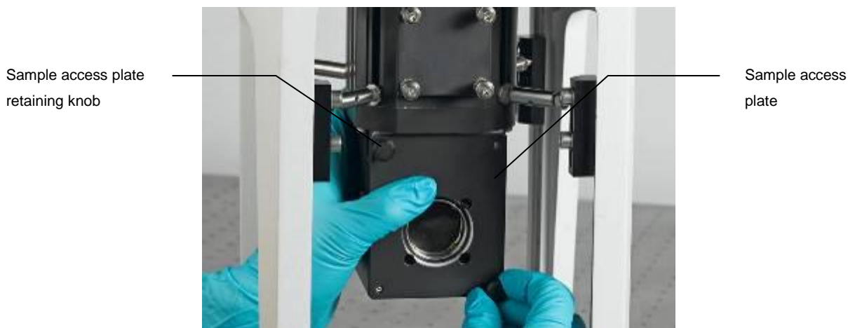
Figure 36 Remove sample access plate
