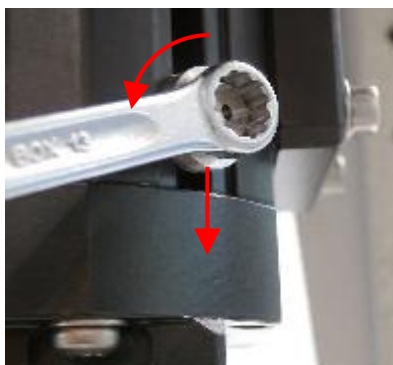
Figure 23 Loosen the locator studs
