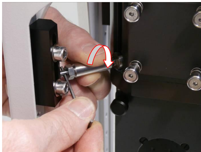
Figure 27 Increase the length of the radial constraints using your fingers
