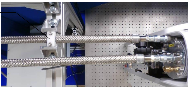
Figure 30 Restrain the supply line without damaging it
