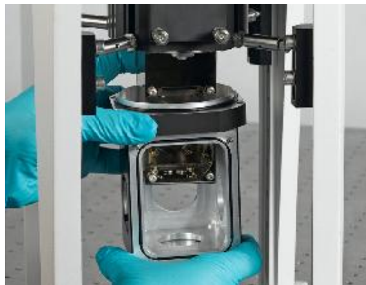
Figure 48 Remove optical window block
