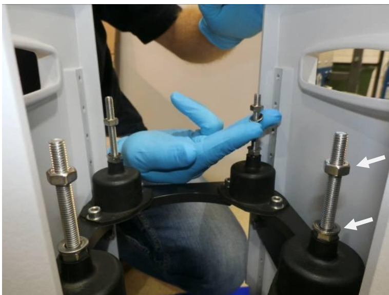
Figure 12 OptistatDry BL4 DRYSTDV support stand anti-vibration mounts
