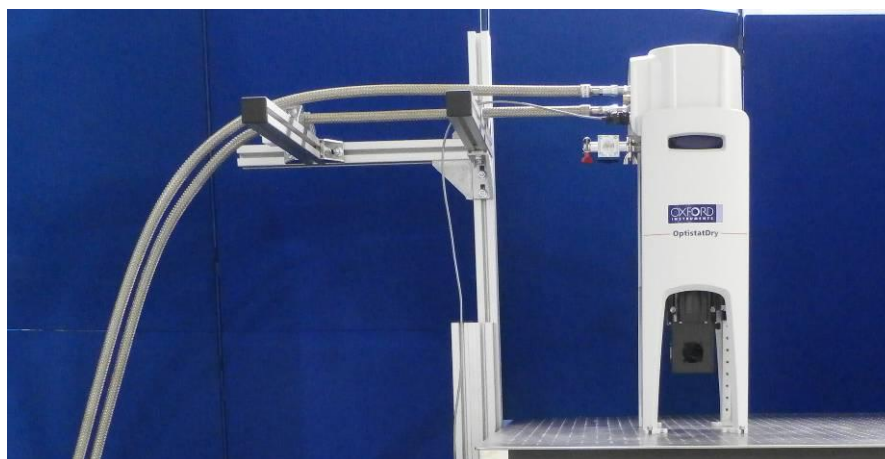
Figure 29 Support the lines horizontally
