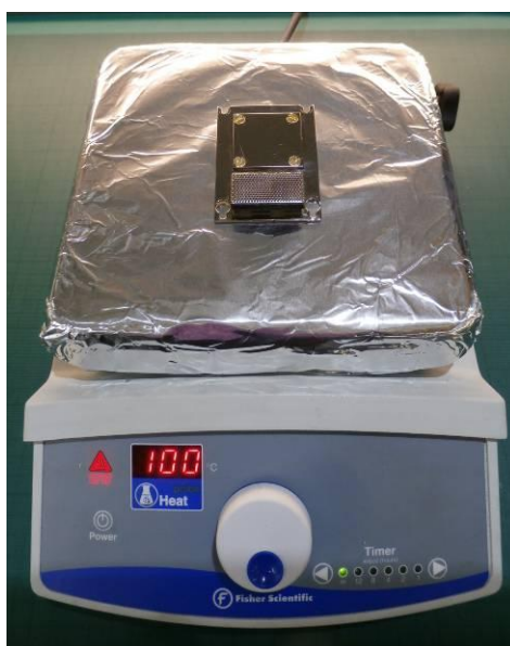
Figure 38 Radiation shield plate with integral sorption pump on laboratory hot plate
