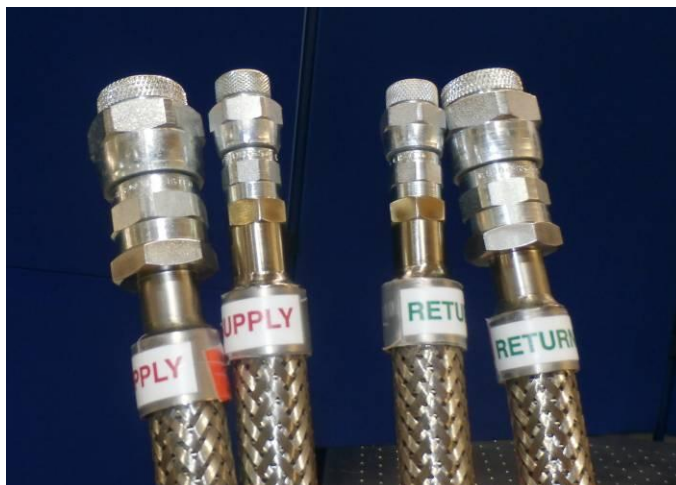
Figure 32 Fit the labels to the lines
