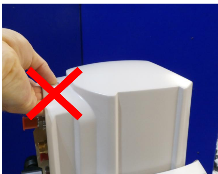
Figure 14 OptistatDry BL4 DRY- do NOT lift from the cover
