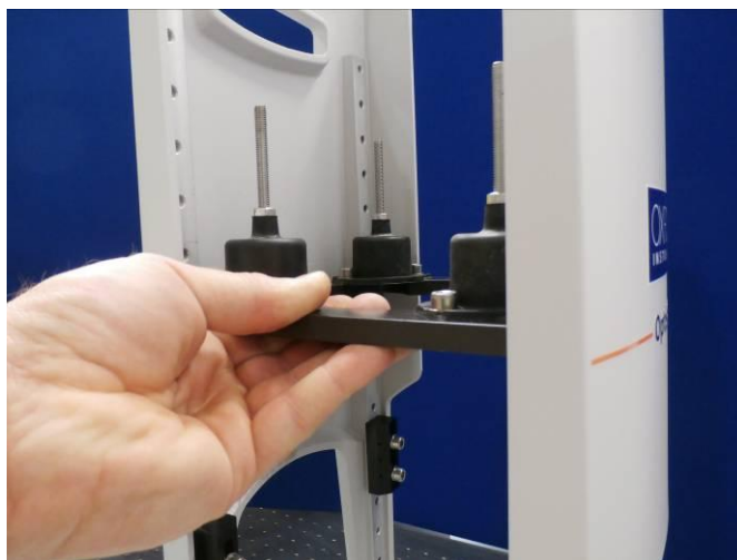
Figure 11 OptistatDry BL4 DRYSTDV support stand cradle adjustment
