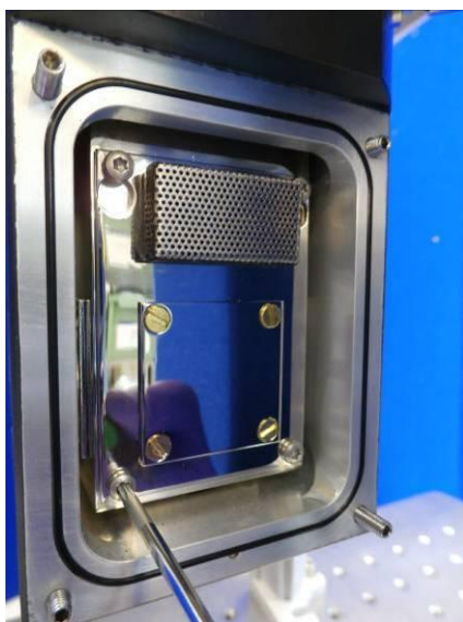
Figure 37 Remove radiation shield plate
