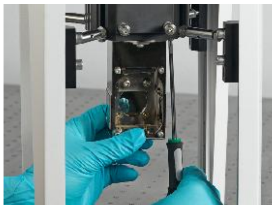
Figure 49 Remove Torx bolts in radiation shield tail
