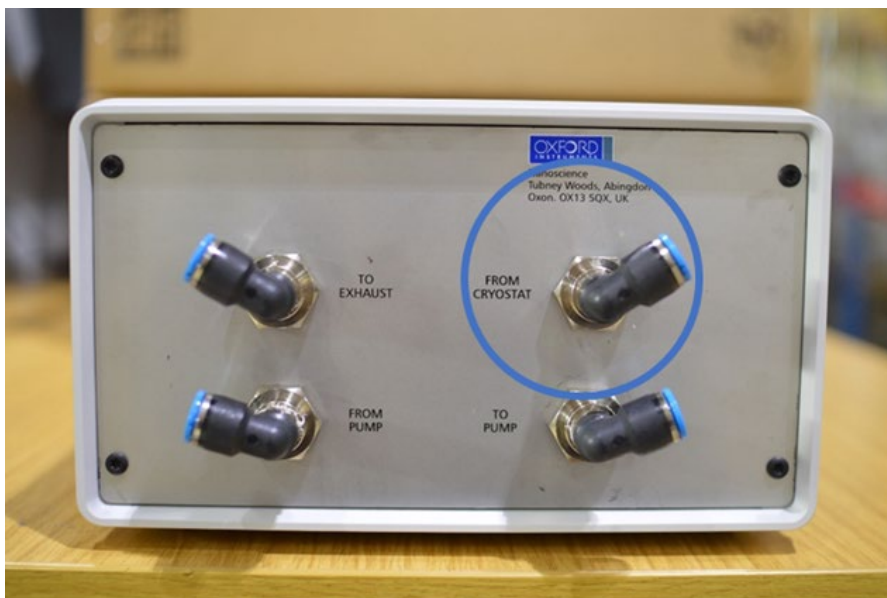
Figure 4-3: Rear view of the VC-U gas flow controller showing the connectors.
