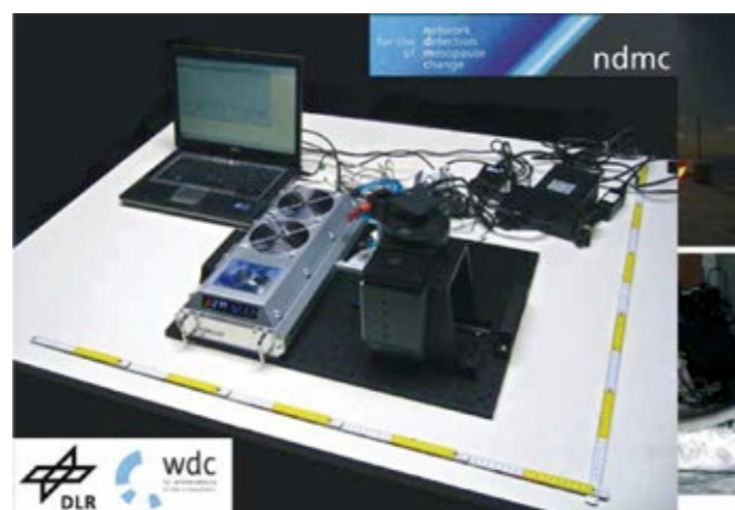
Figure 1: Setup of the GRIPS 6 instrument at the German Remote Sensing Data Center in Oberpfaffenhofen (48.09°N / 11.28°E). The instrument is composed of an Andor Shamrock 163 spectrograph, an Andor iDus DU490A-1.7 photodiode array, powered by a PS-25 power supply for deep cooling temperatures in combination with an Exos-2 water recirculator. The laptop shows a 15 s exposure of the OH nightglow between 1500 to 1600 nm obtained with the Andor Solis software.
