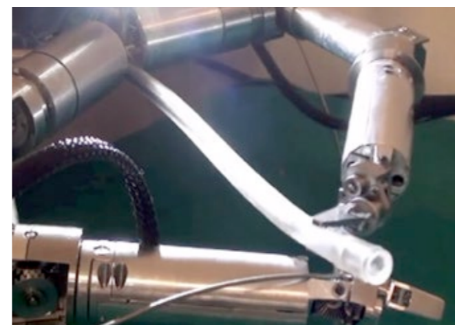
Figure 2: The fiber probe being held and manipulated by the robotic arm of ARAKNES.
