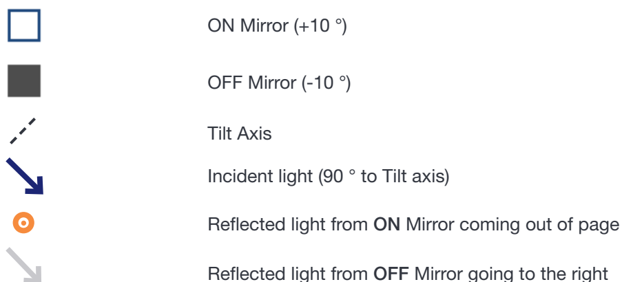
Figure 4: A representation of a small area of a DMD Mirror array (face-on view)
