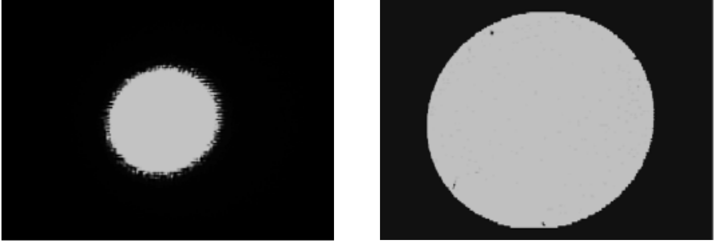
Figure 16: (left) Small but poorly focused spot, (right) Larger but sharply focused spot
