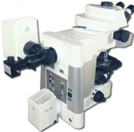
Figure 2-1: Schematic of a Manual MicroPoint Laser Illumination and Ablation System Installed on an Upright Microscope
