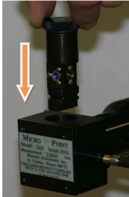
Figure 4-2: Inserting the Dye Cell into the Resonator Block.
