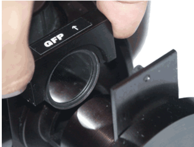
Figure 3-5: Lamp House Filter Installation
