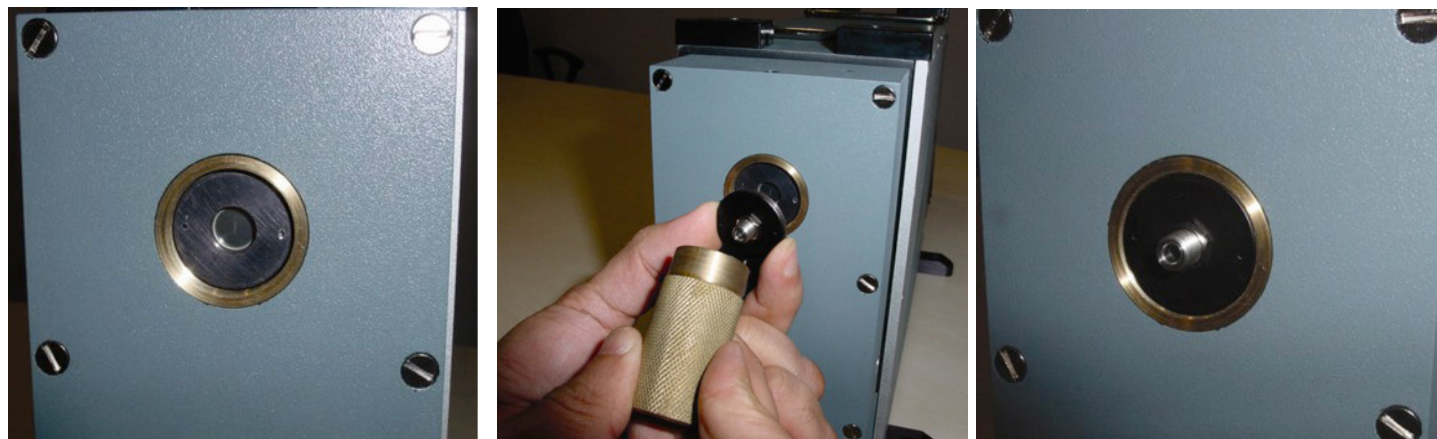
Figure 27: Fitting an SMA connector over the slit disc using the brass insertion tool
