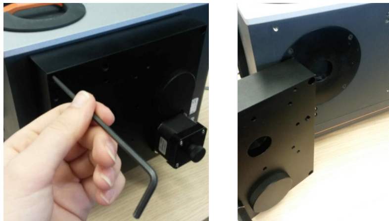
Figure 8: Removal of the filter wheel (left), once removed the shutter can be accessed (right).
